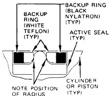
TYPICAL ACTIVE DYNAMIC SEAL ASSEMBLY INSTALLATION
