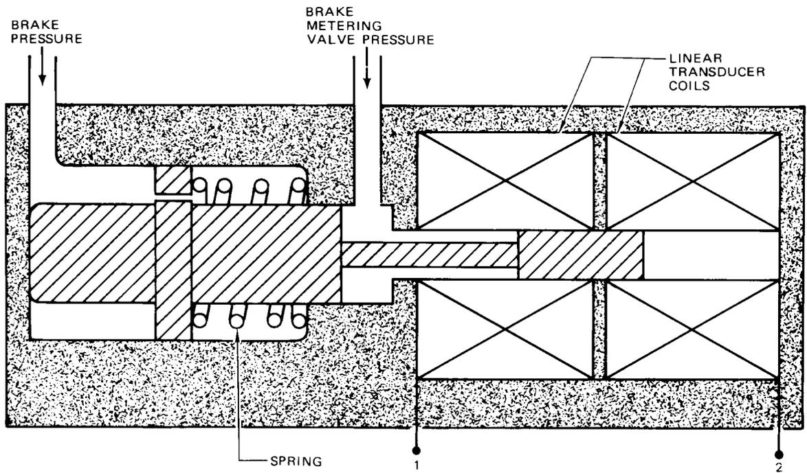
Brake Pressure Comparator Schematic
