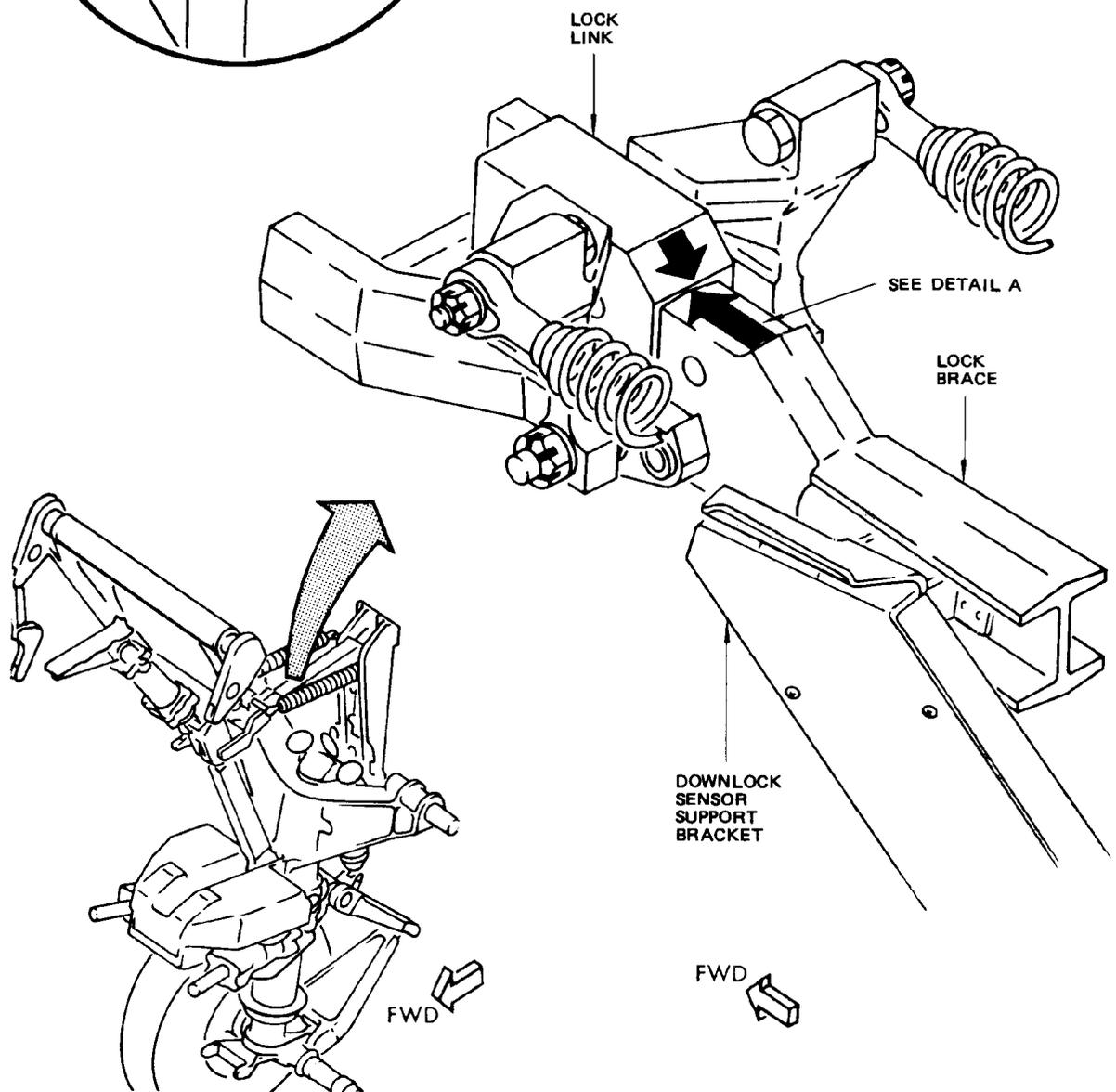
Nose Landing Gear Mechanical Downlock Indication
