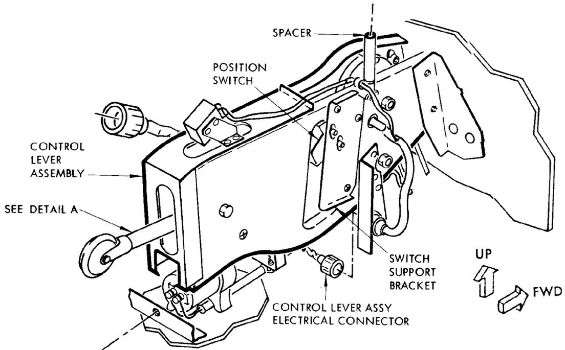
Control Lever Position Switch Installation
