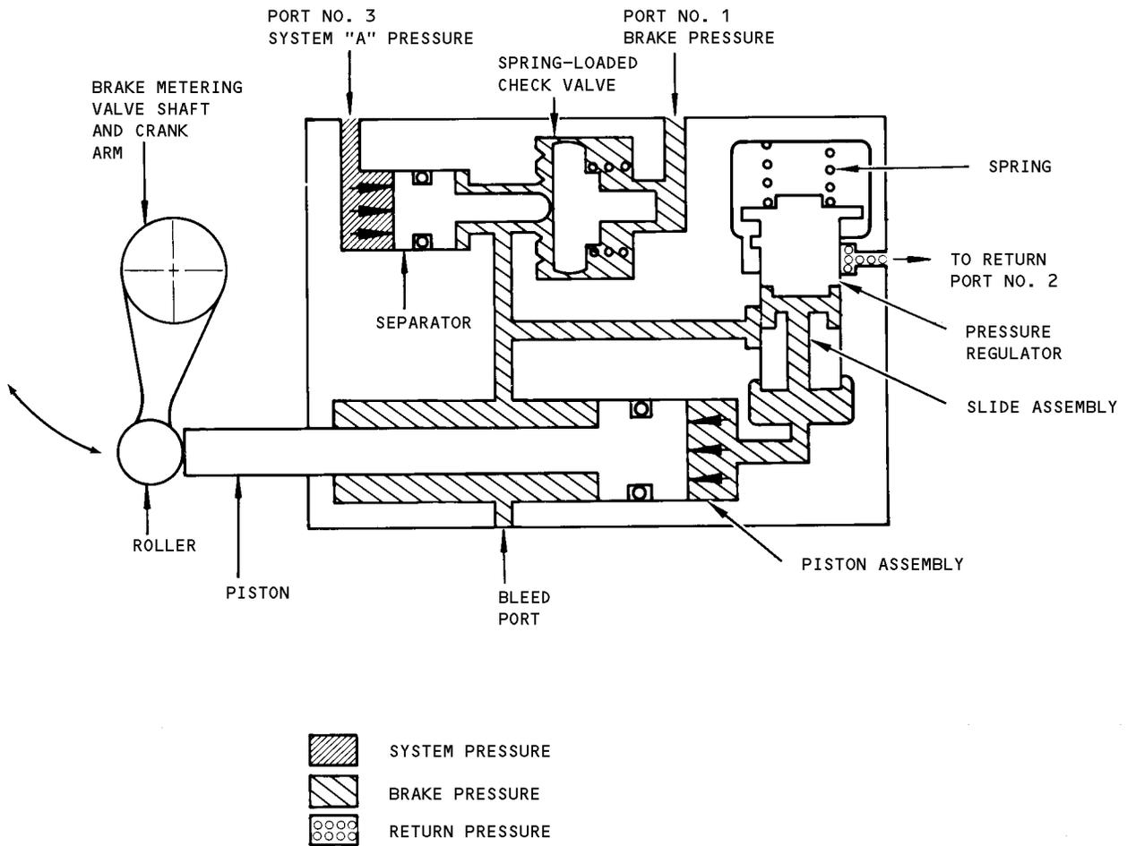
Brake Valve Feel Augmentation Actuator Schematic
