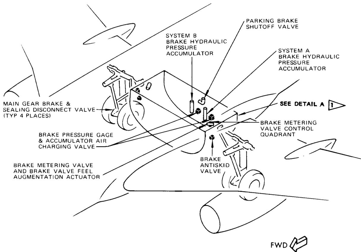
Brake Hydraulic System Component Location
