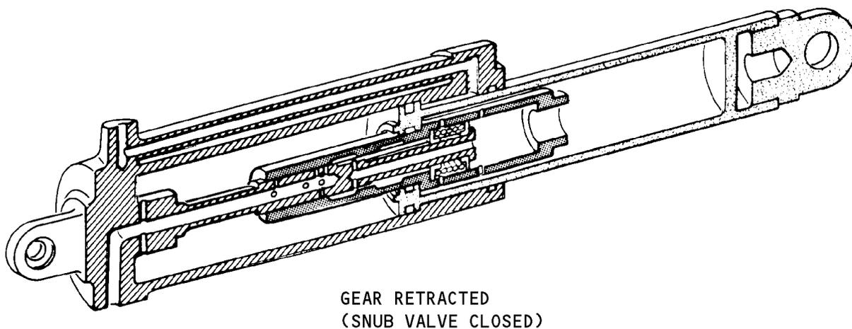
Main Gear Actuator Schematic
