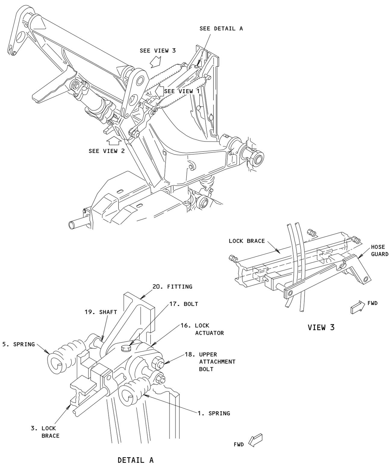
Nose Gear Lock Mechanism Installation
