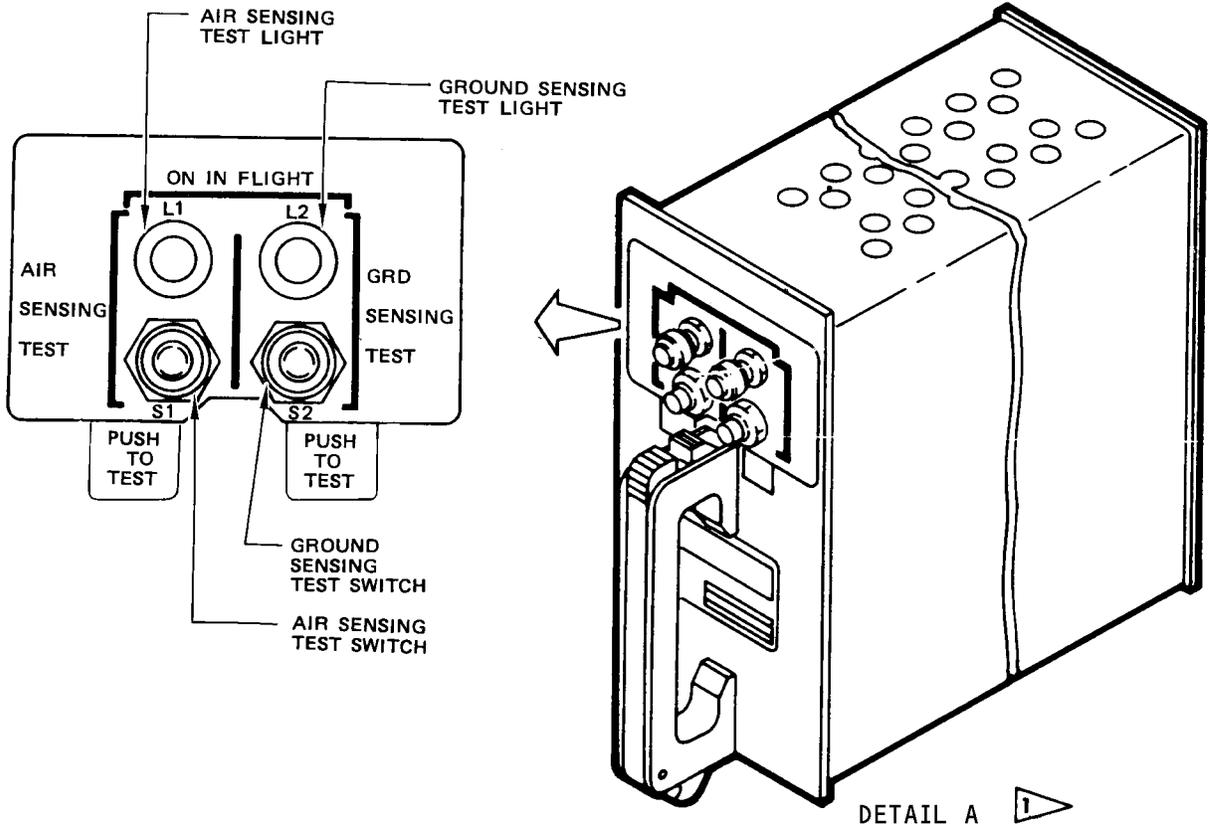
Landing Gear Electrical Module
