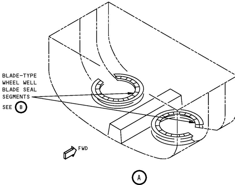
Main Landing Gear Wheel Well Blade Seal - Inspection/Check
