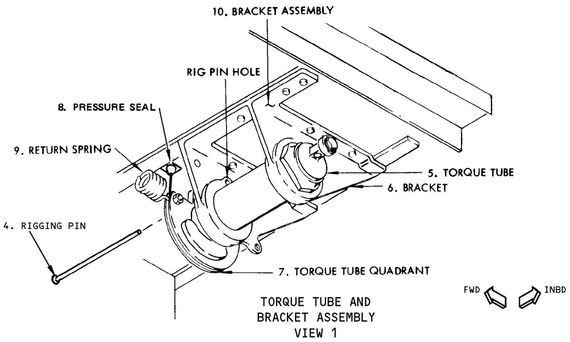
Nose Gear Manual Extension System Cable Removal/Installation
