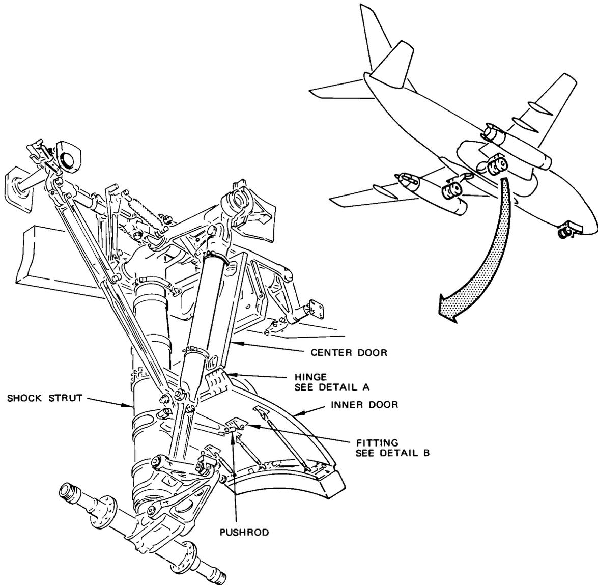
Main Gear Shock Door Wear Limits
