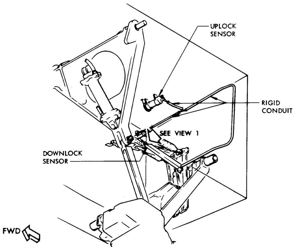
Downlock Sensor and Sensor Actuator Installation
