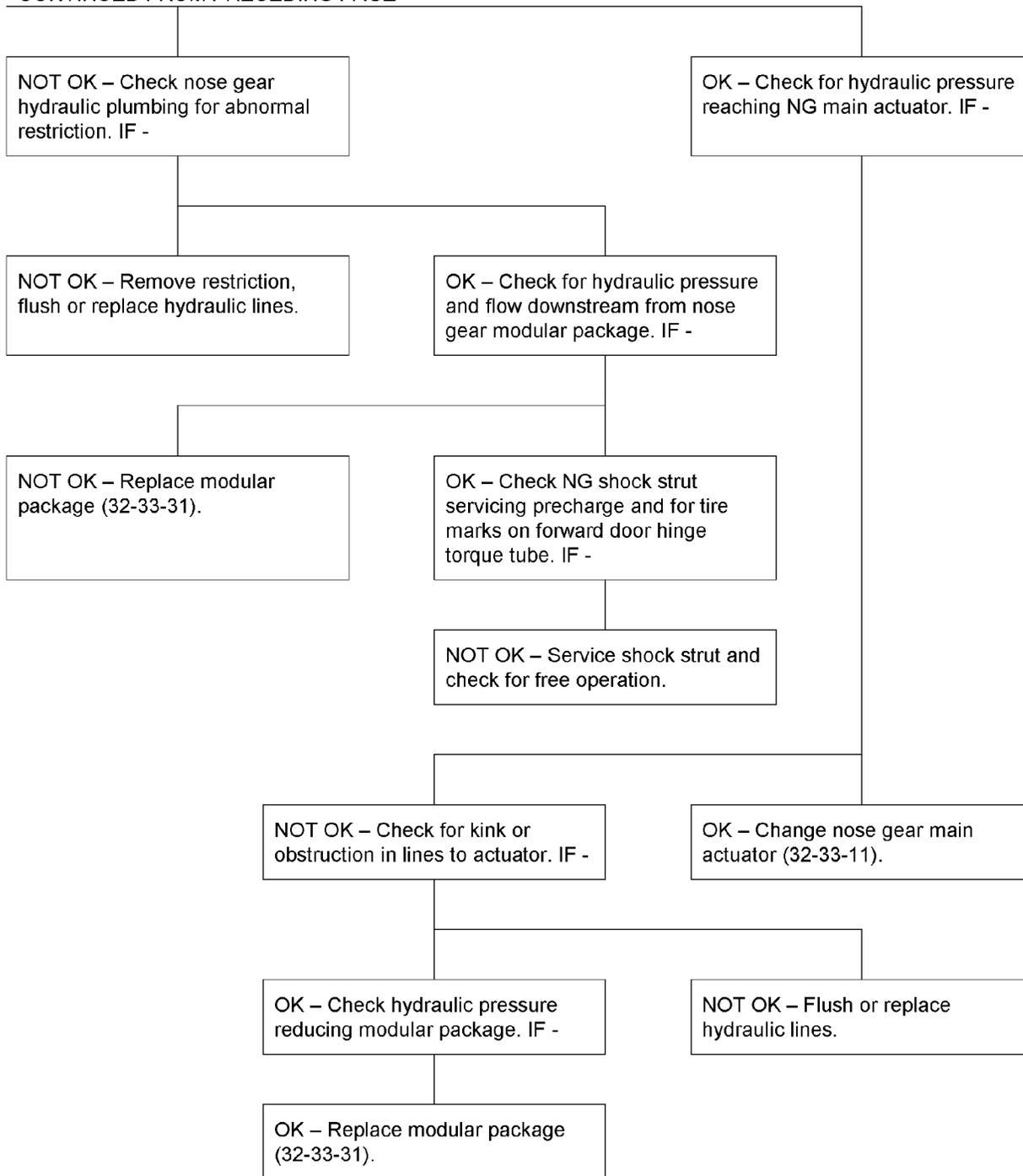
Testing and Fault Isolation
