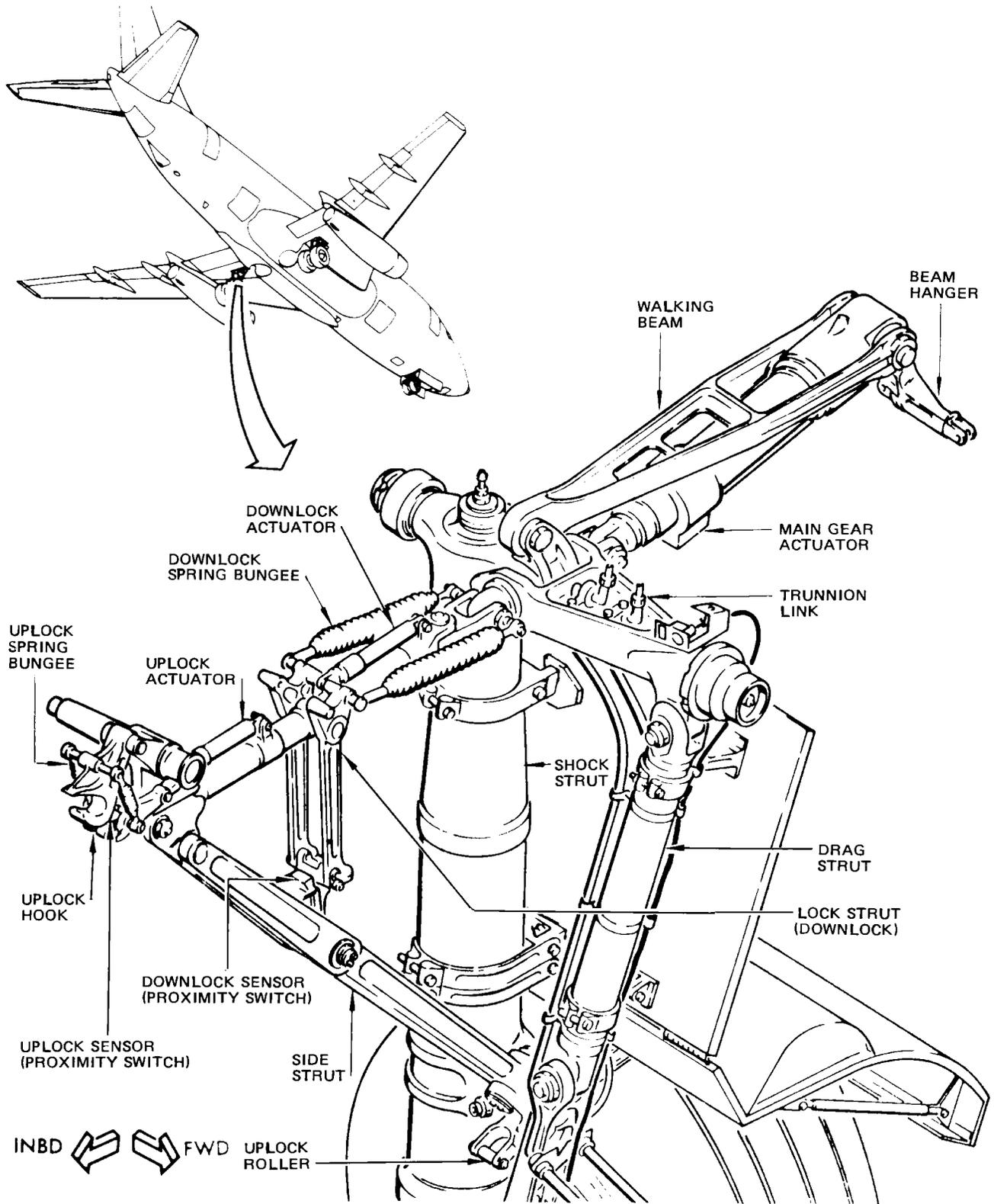
Main Gear Extension and Retraction Components Locations
