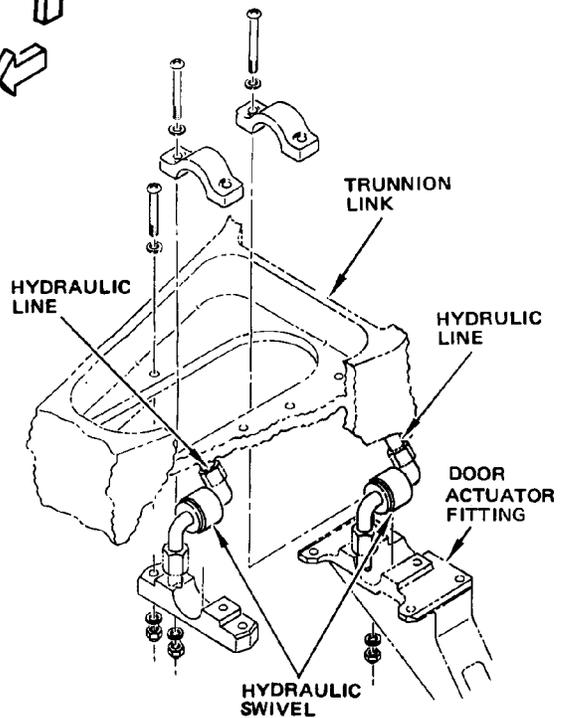
Main Gear Hydraulic Lines and Electrical Cables
