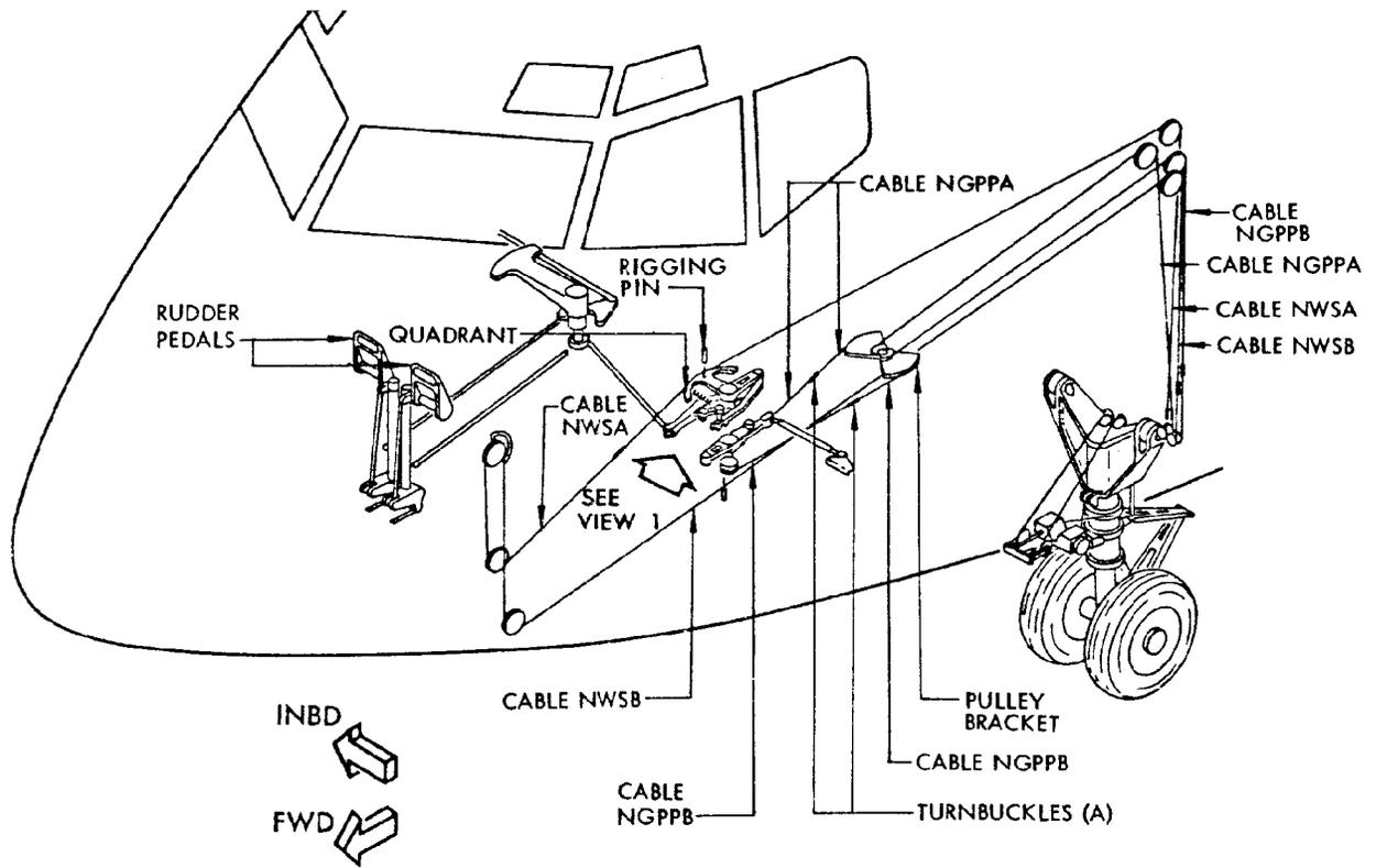
Rudder Pedal Steering Mechanism Installation
