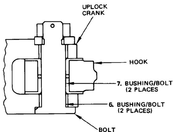
Main Gear Uplock Mechanism Wear Limits
