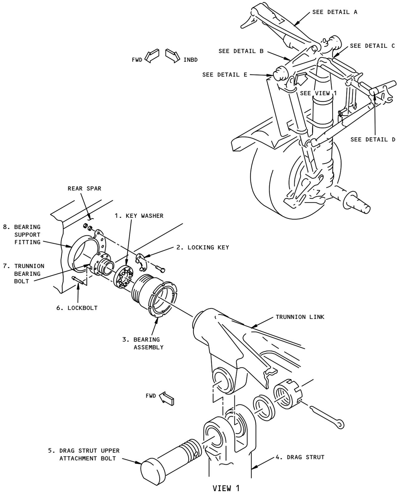
Main Gear Trunnion Link Installation
