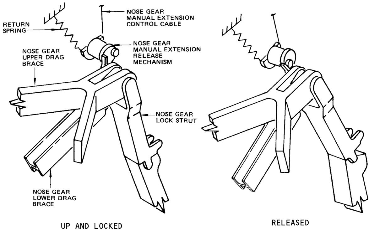
Nose Gear Manual Extension System Component Location
