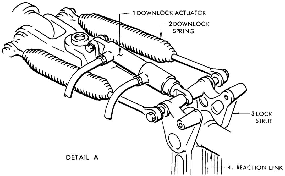
Main Gear Reaction Link Installation
