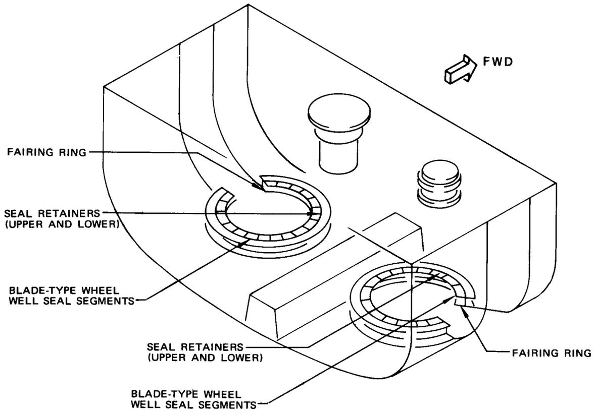
Main Gear Wheel Well Seal Component Location
