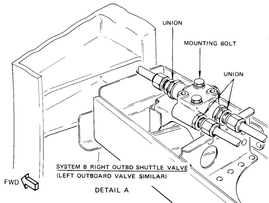
Autobrake Shuttle Valve Installation
