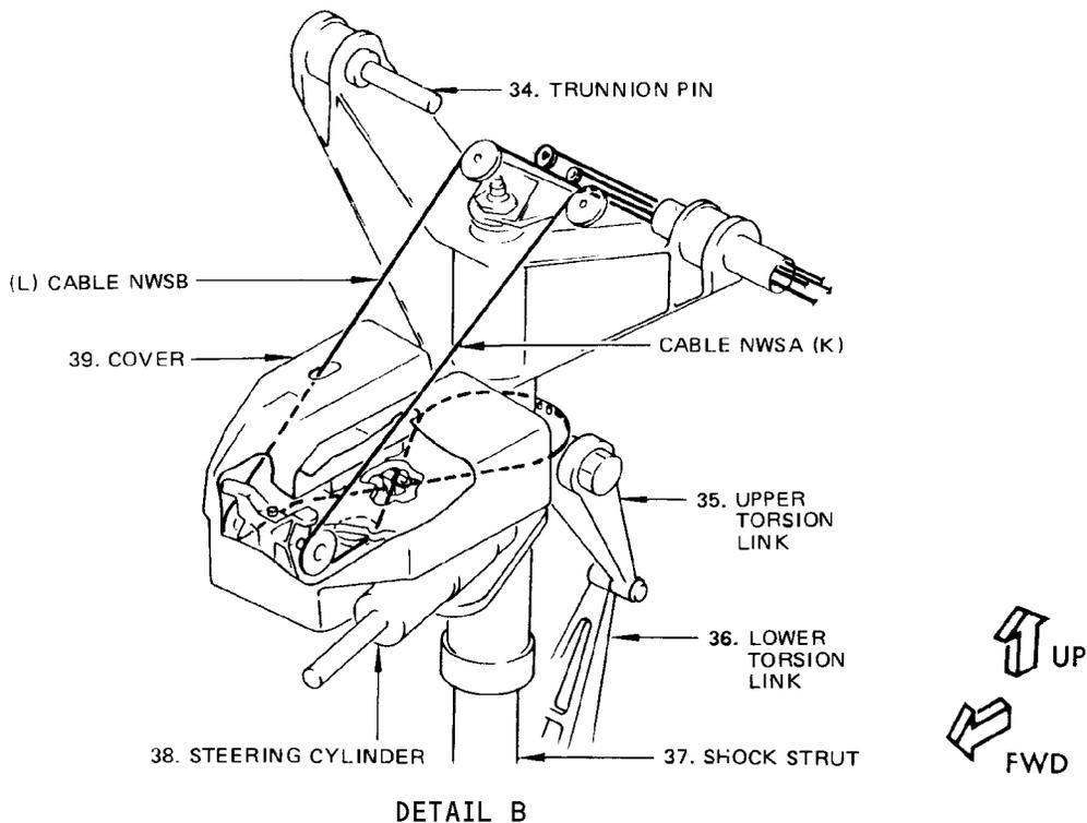
Steering System Cables Removal/Installation
