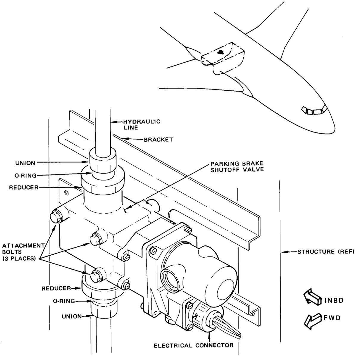
Parking Brake Shutoff Valve Installation
