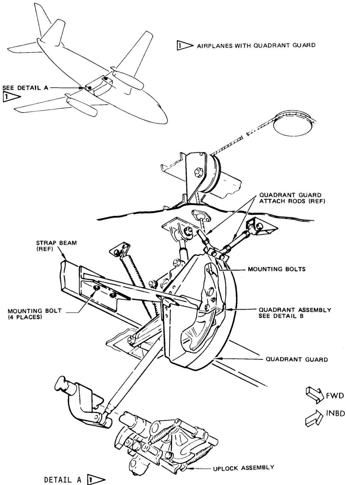
Main Gear Manual Extension Linkage Installation
