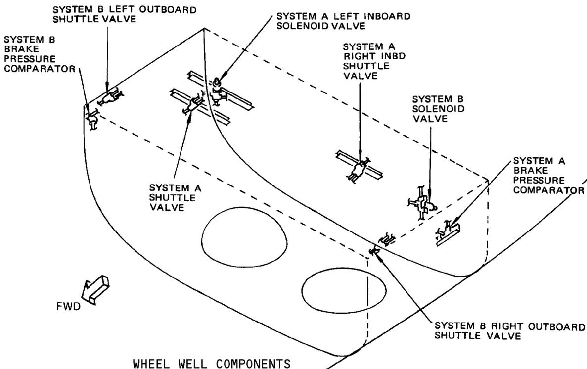
Automatic Braking System Component Locations
