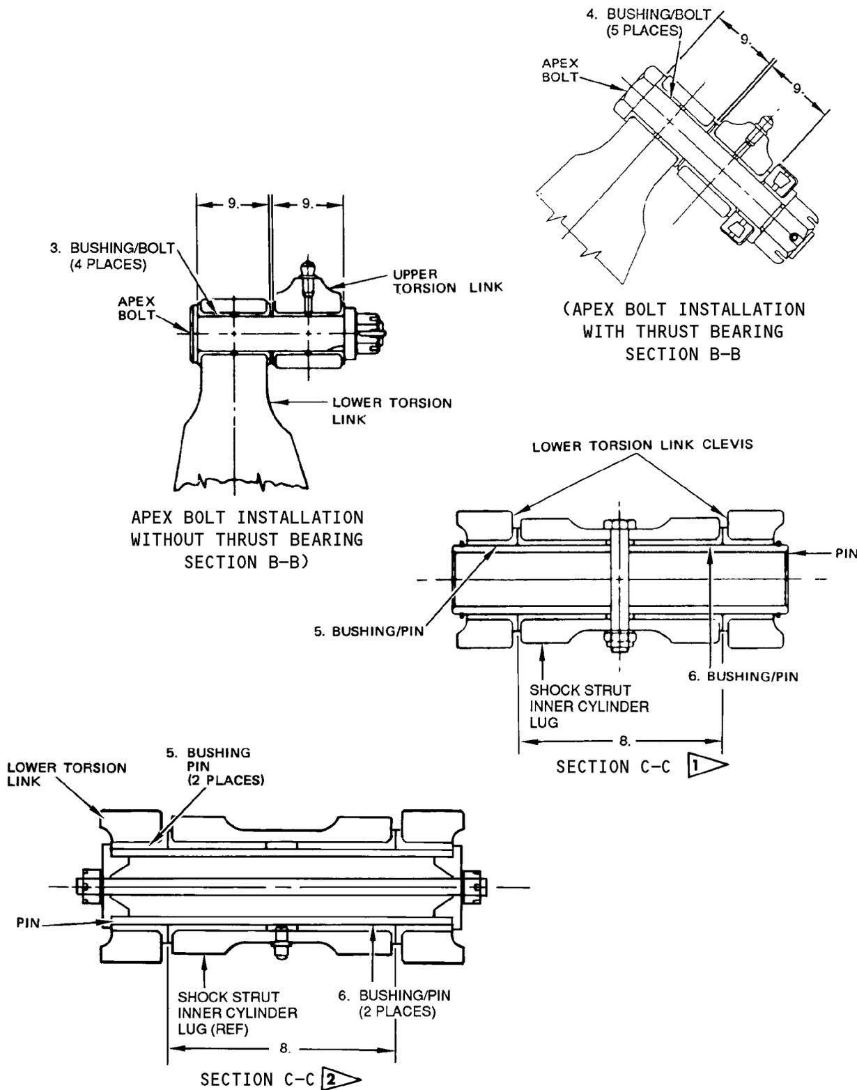
Nose Gear Torsion Links Wear Limits
