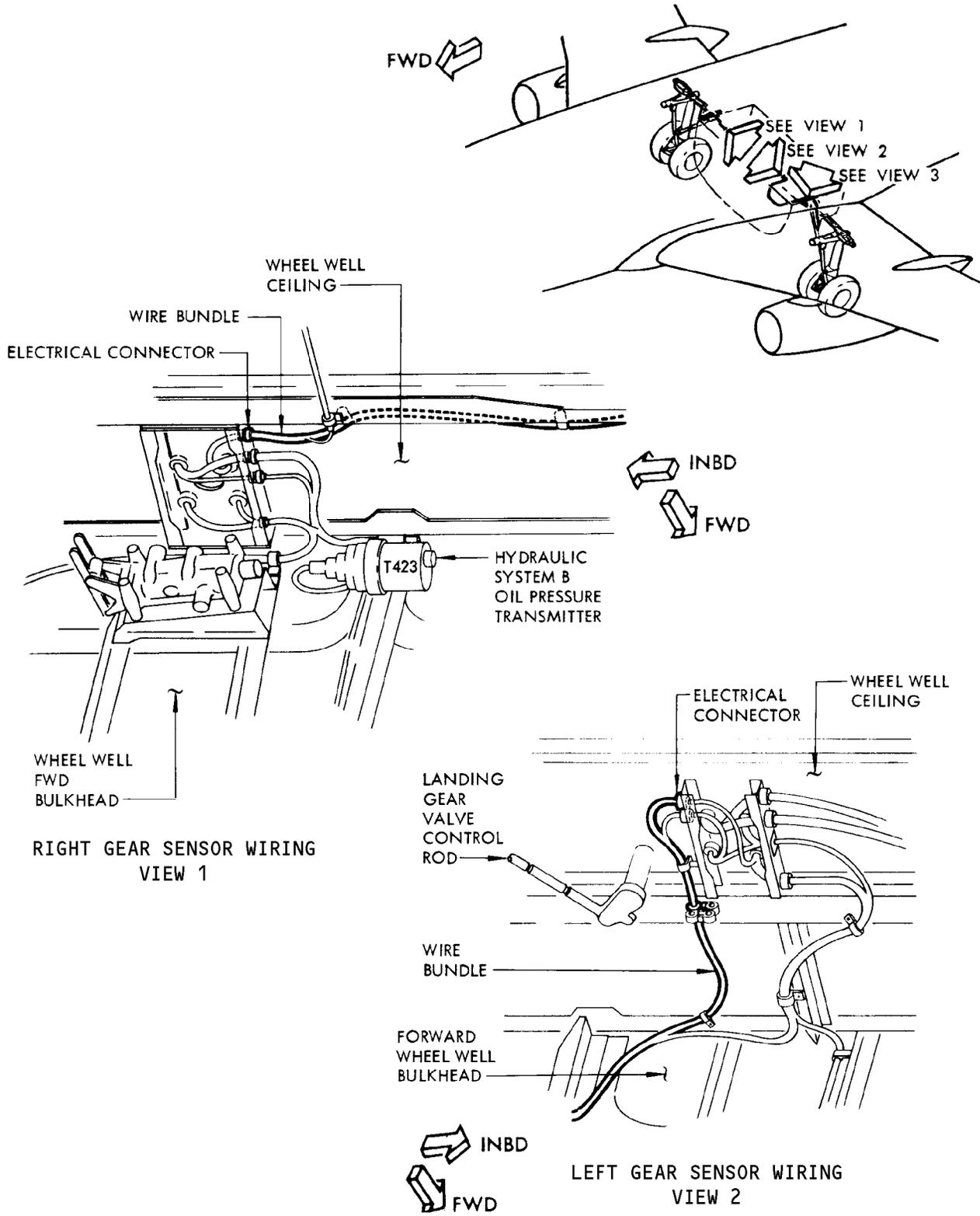
Main Gear Downlock Sensor Installation
