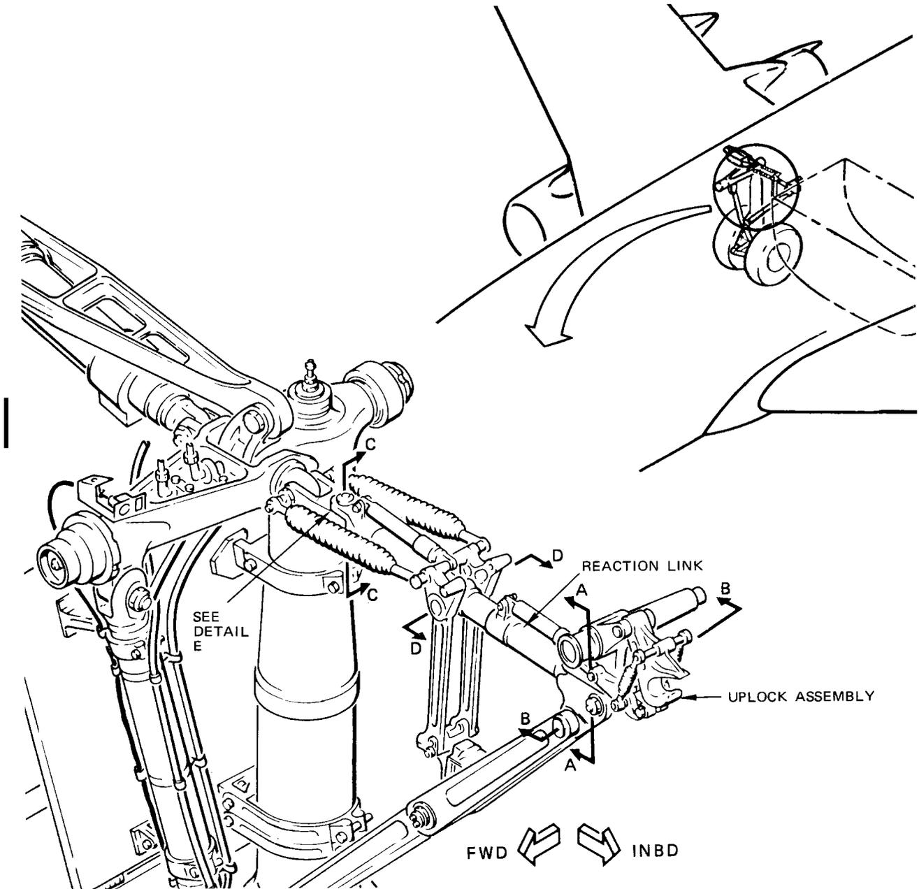
Main Gear Reaction Link Wear Limits
