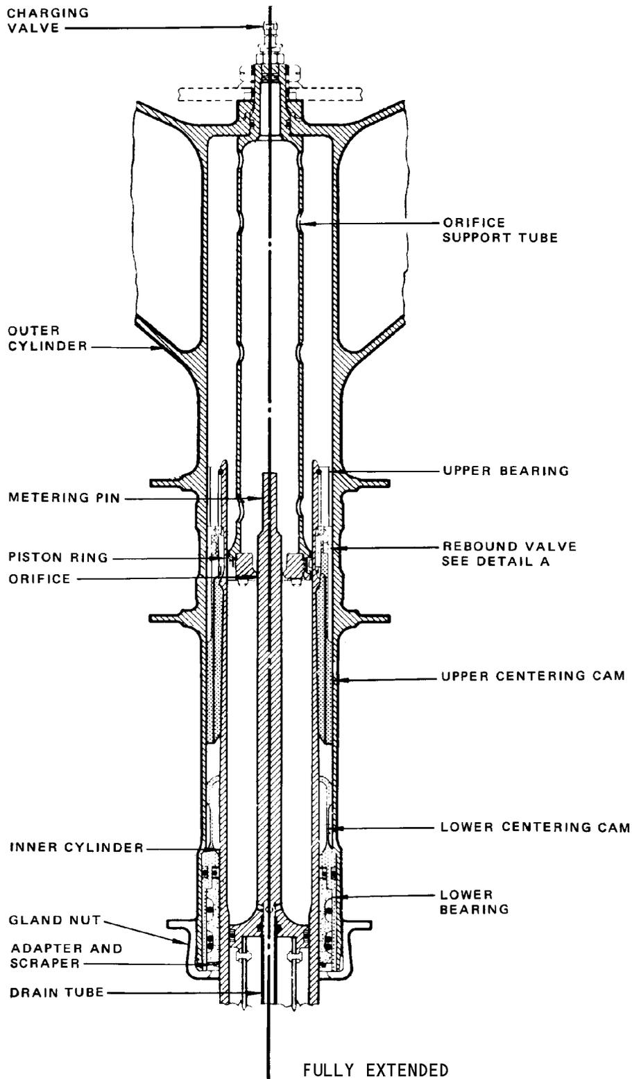
Nose Gear Shock Strut Schematic
