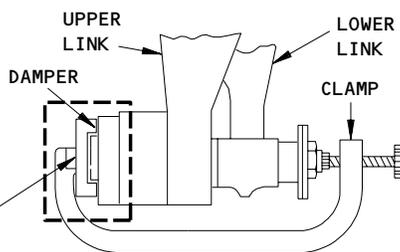
**NOTE:** LOCATE CLAMP ON DAMPER BODY. USE SOCKET OR WOODEN BLOCK WITH HOLE IF NECESSARY
