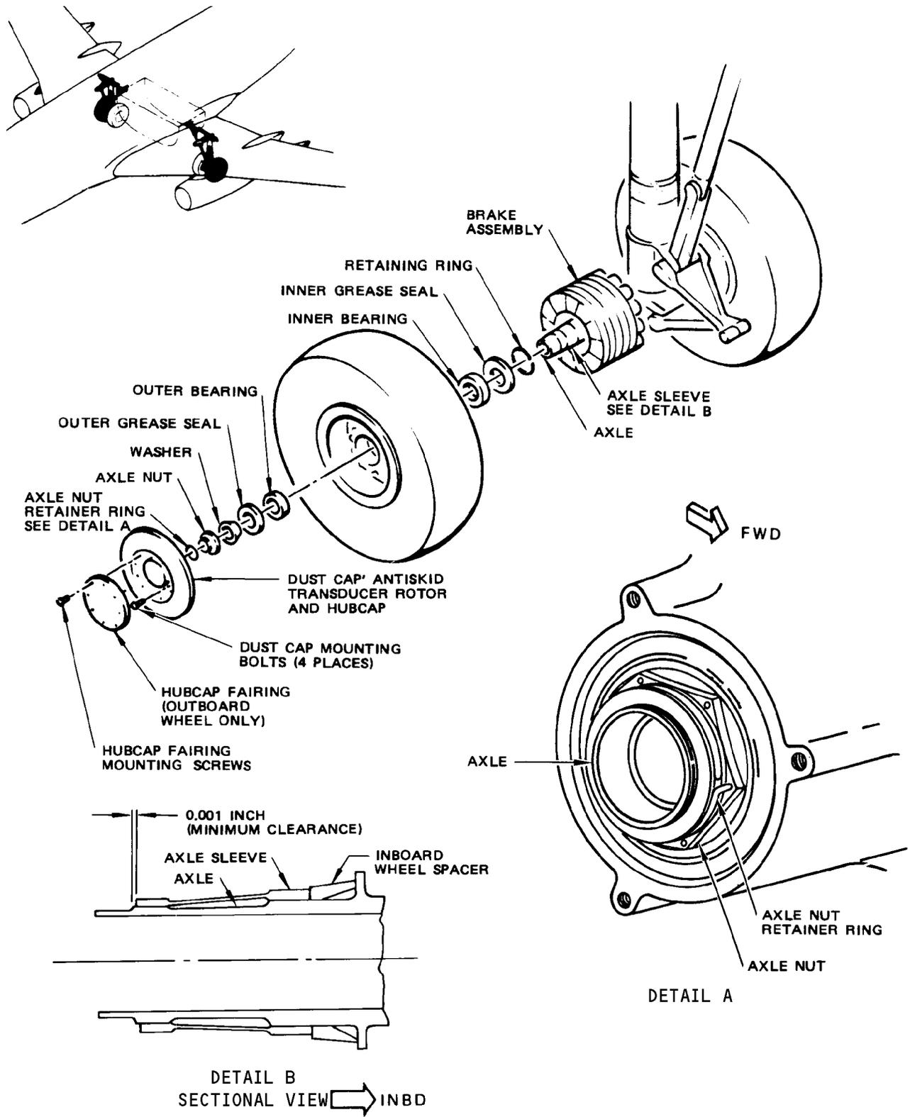
Main Gear Wheel Installation
