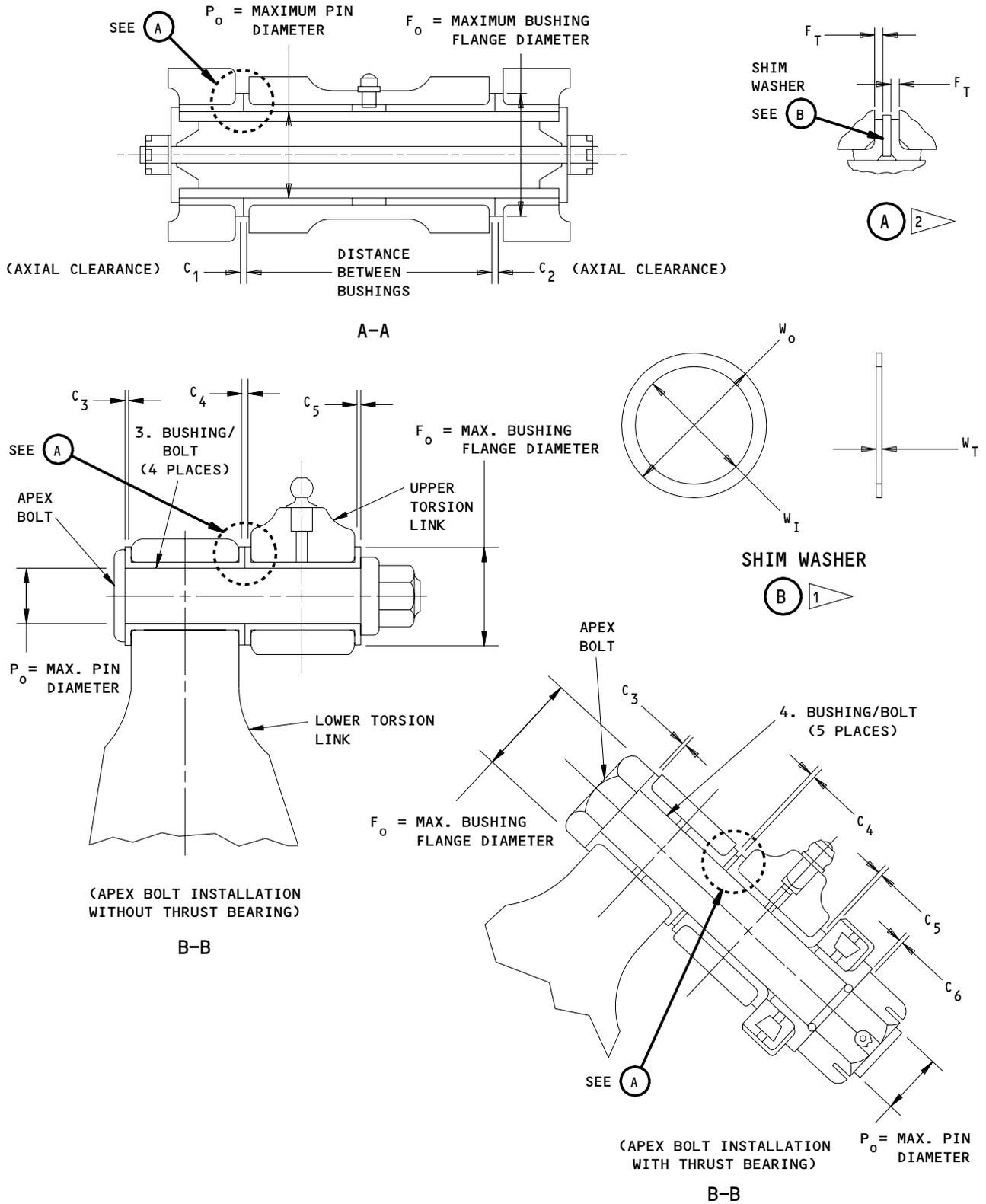
Special Repairs - Shim Axial Clearance
