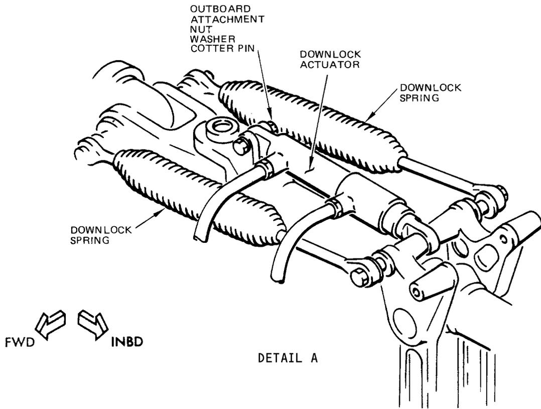
Main Gear Downlock Actuator Installation
