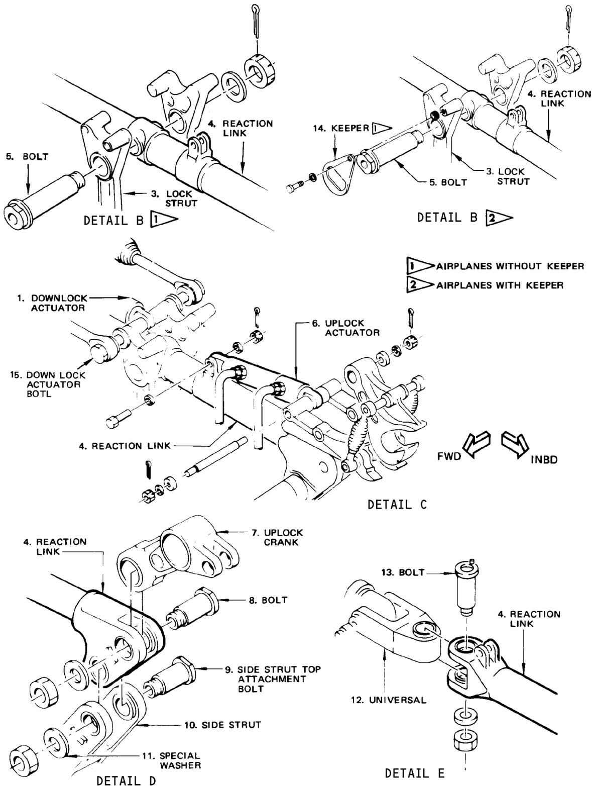
Main Gear Reaction Installation
