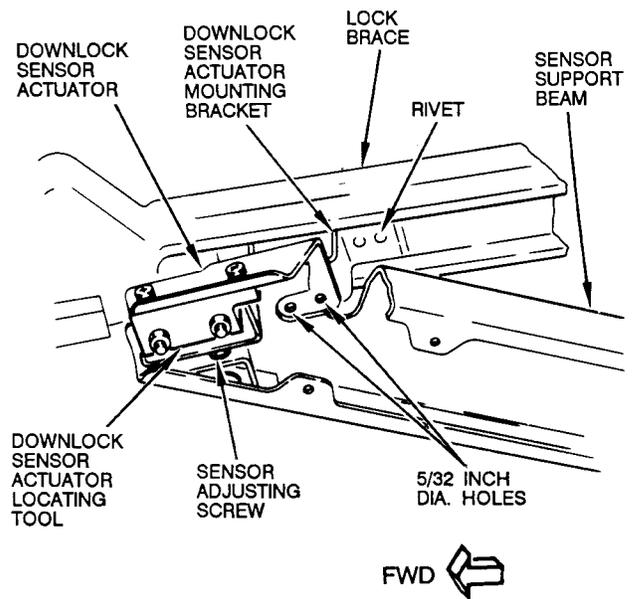
SENSOR ACTUATOR INSTALLATION
