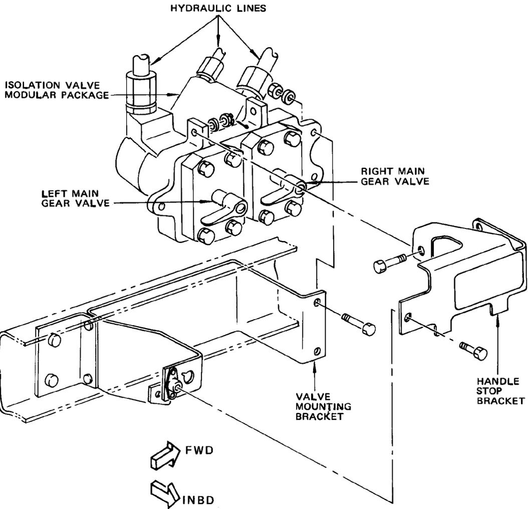
Main Gear Isolation Valves, Modular Package Installation
