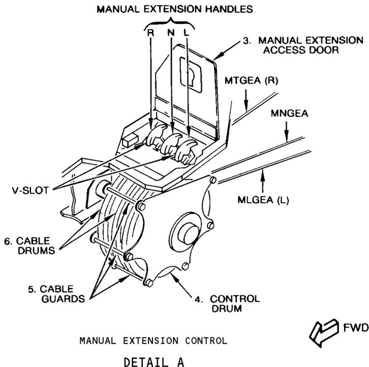
Main Gear Manual Extension System Cable Installation
