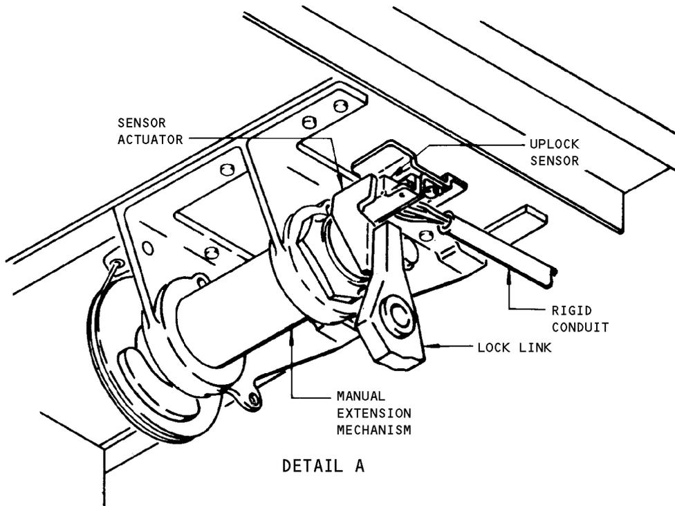
Nose Gear Uplock Sensor Adjustment
