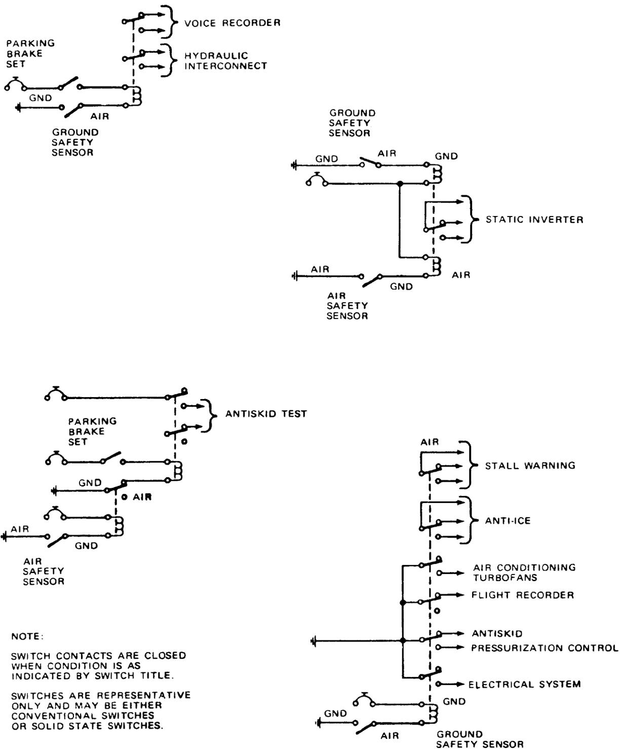
Air-Ground Sensing Functional Schematic
