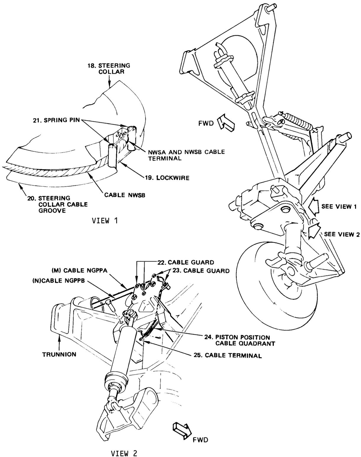
Steering System Cables Installation
