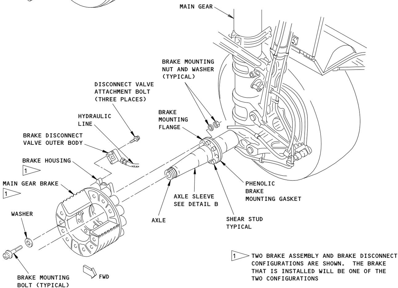
**INSTALLATIONS WITH PHENOLIC BRAKE MOUNTING GASKET**
