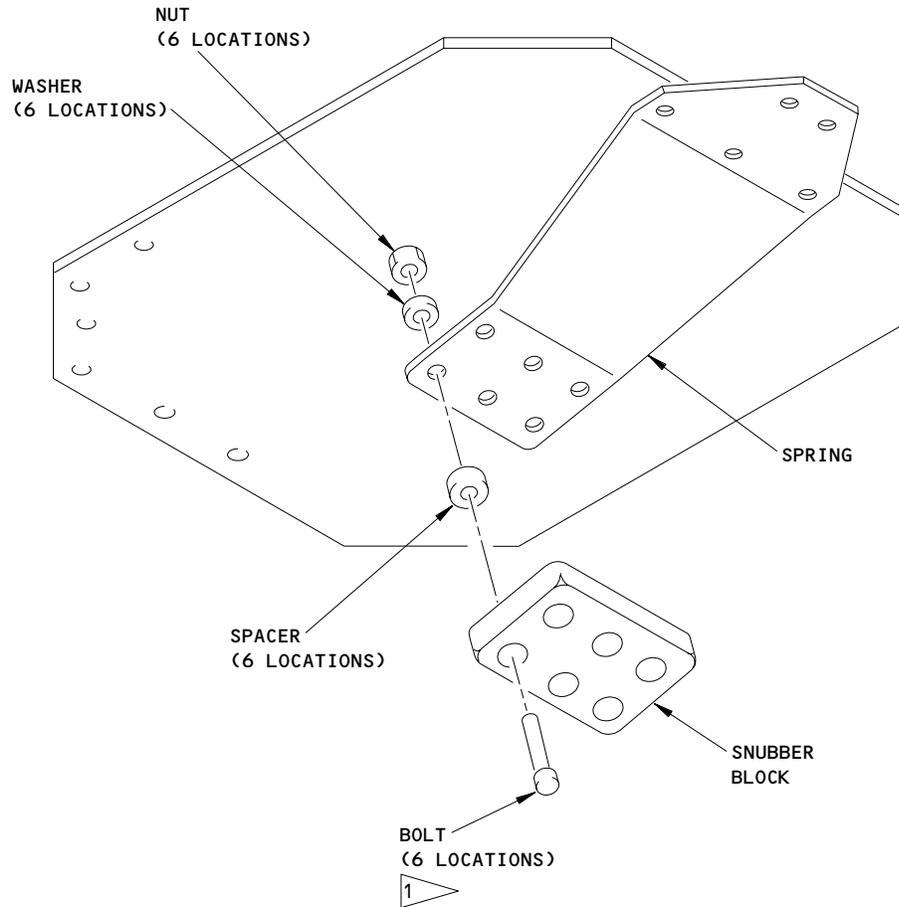
1 FOR ONE OR TWO SPACERS, 1-INCH BOLTS ARE USED. IF THREE SPACERS ARE REQUIRED, 1.25-INCH BOLTS MUST BE USED.
