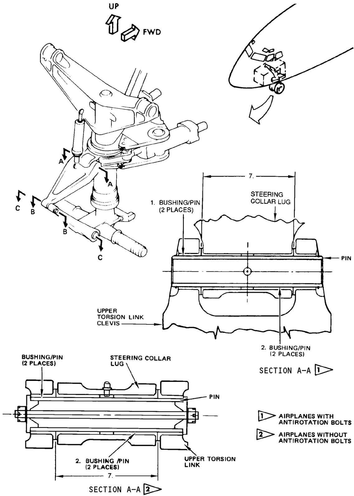
Nose Gear Torsion Links Wear Limits
