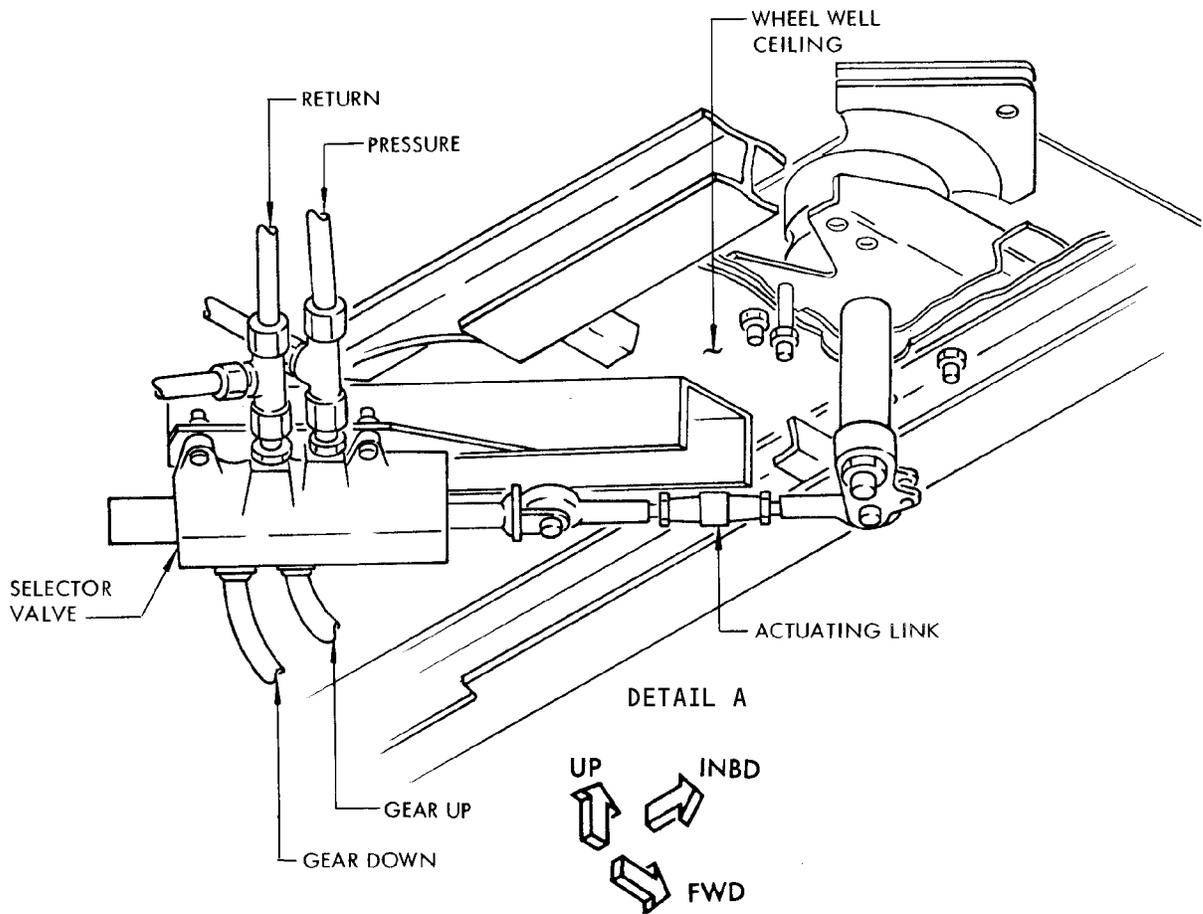
Landing Gear Selector Valve Installation
