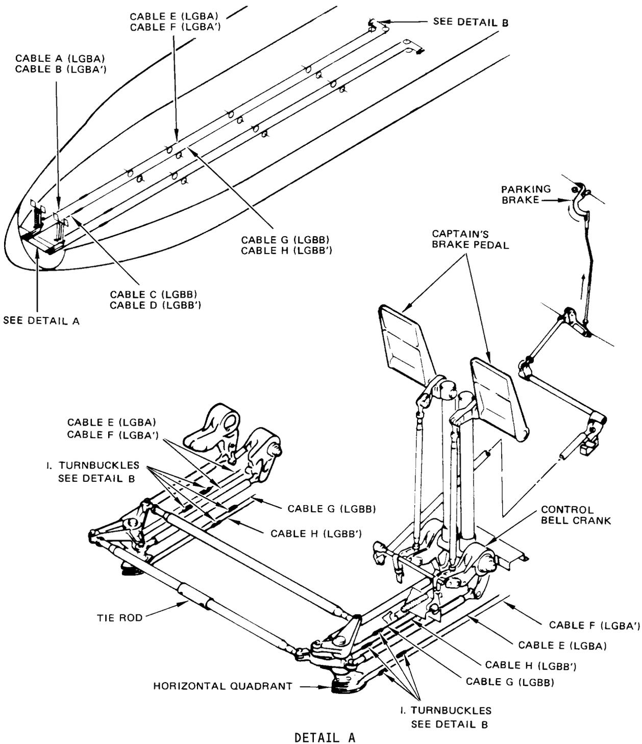
Brake Control Cables Installation
