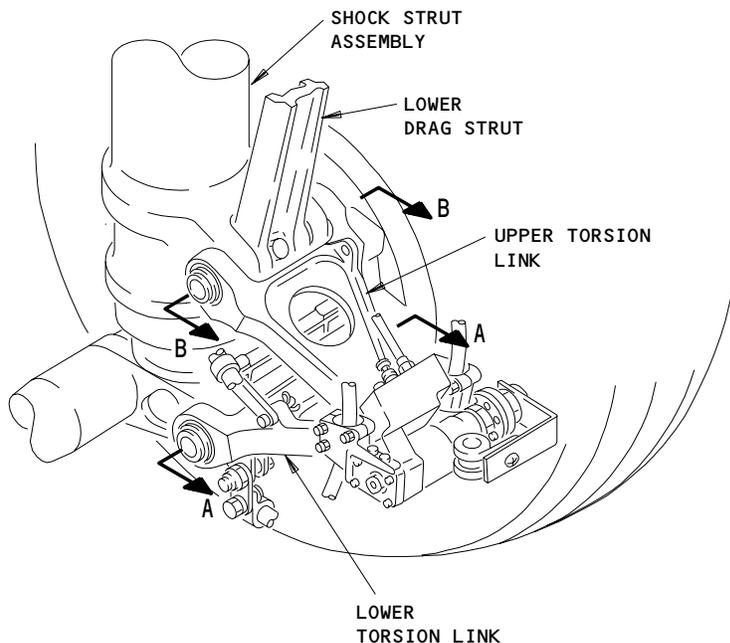
MAXIMUM AXIAL CLEARANCE  $\triangle 3 = C_T = C_1 + C_2$
