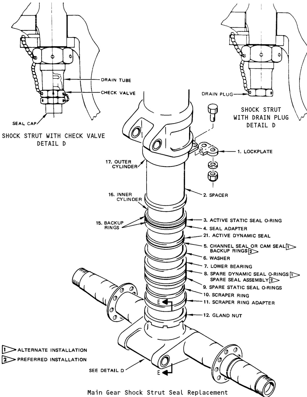
Main Gear Shock Strut Seal Replacement
