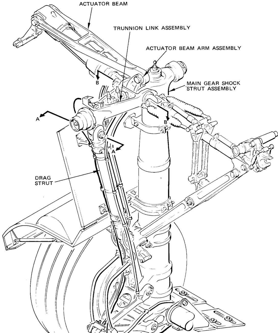
Main Gear Trunnion Assembly Wear Limits
