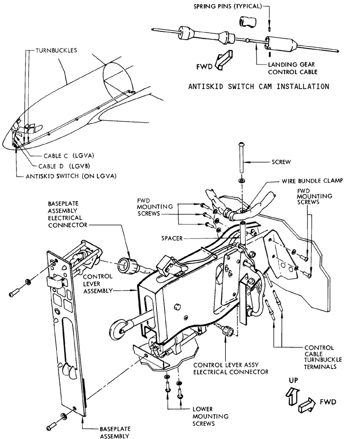
Landing Gear Control Lever Installation
