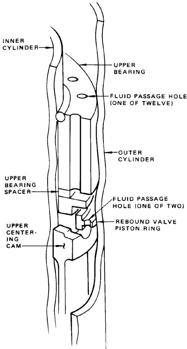
STATIC POSITION OF REBOUND VALVE PISTON RING
