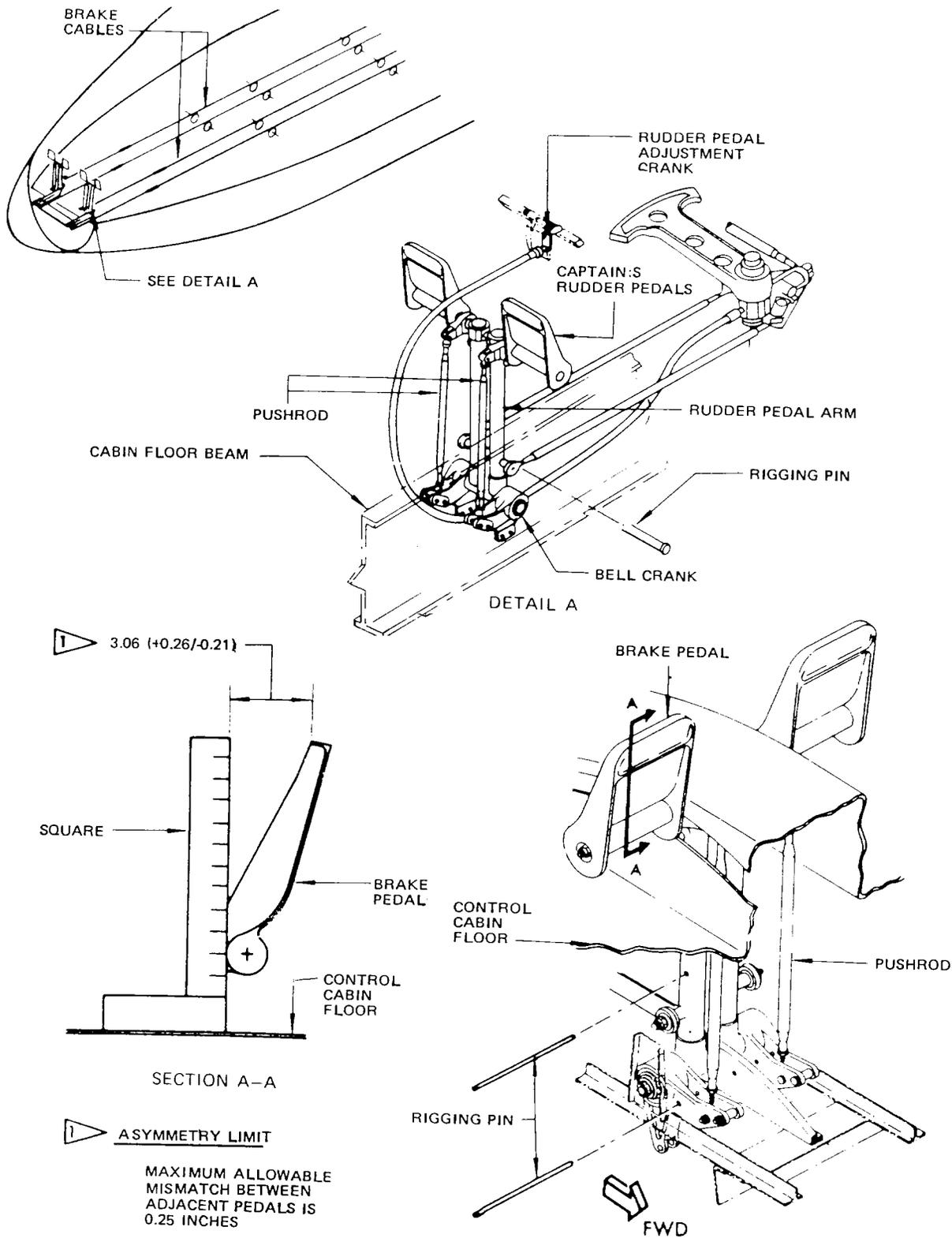
Hydraulic Brake Pedal Adjustment
