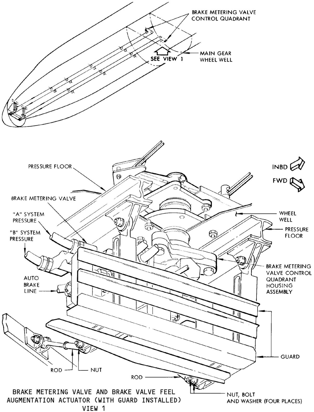
**BRAKE METERING VALVE AND BRAKE VALVE FEEL AUGMENTATION ACTUATOR (WITH GUARD INSTALLED)**
