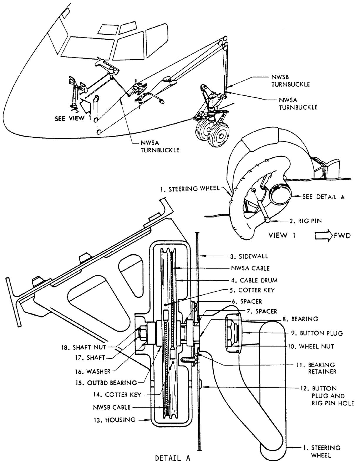
Steering Wheel and Cable Drum Installation
