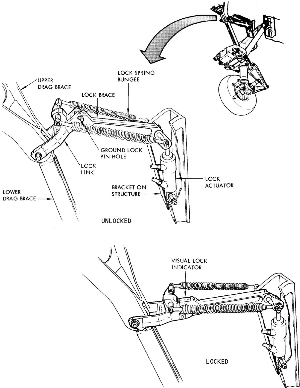
Nose Gear Lock Mechanism
