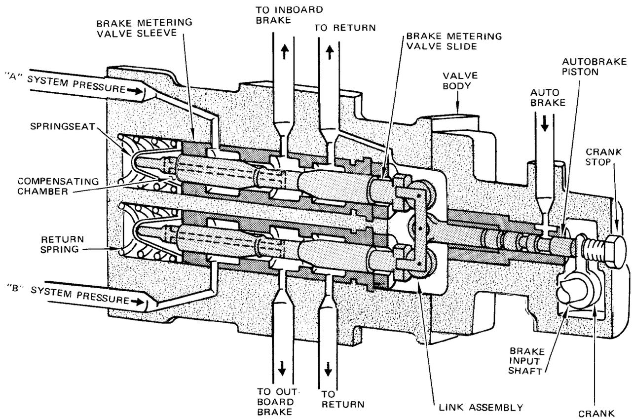
Brake Metering Valve Schematic
