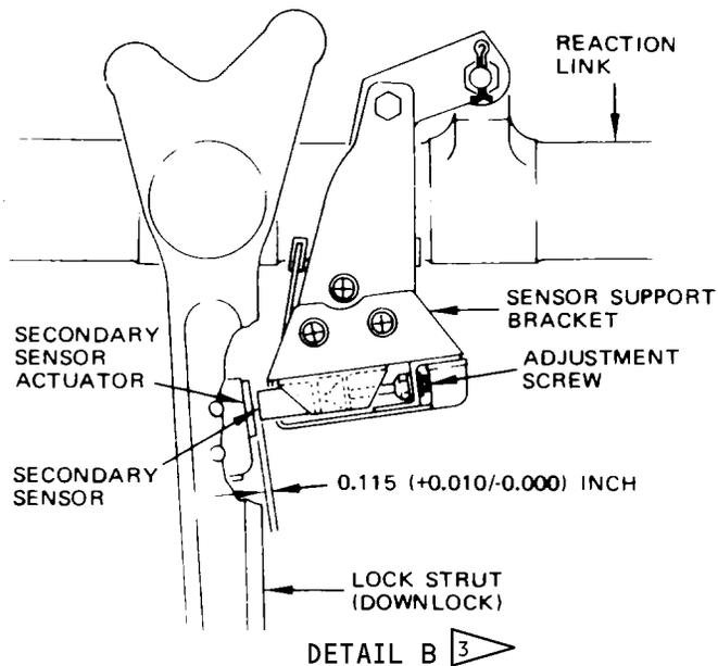
Main Gear Downlock Sensor Installation
