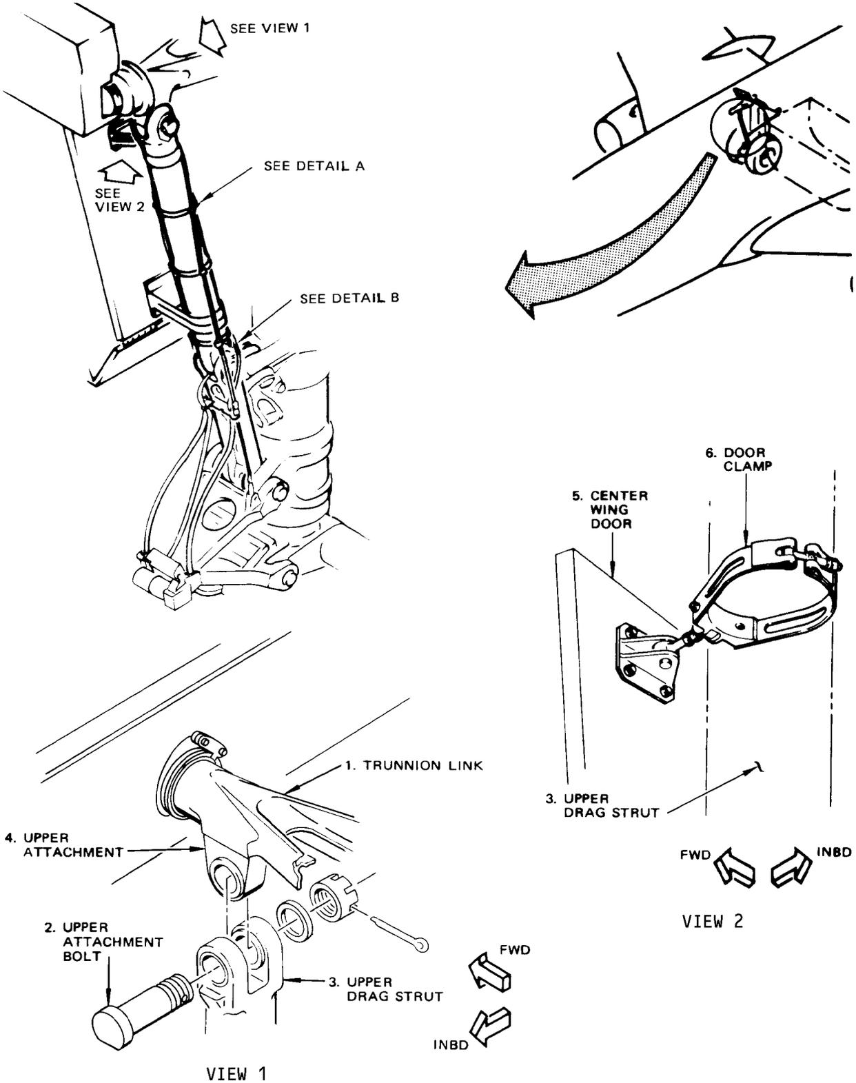
Main Gear Upper Drag Strut Installation
