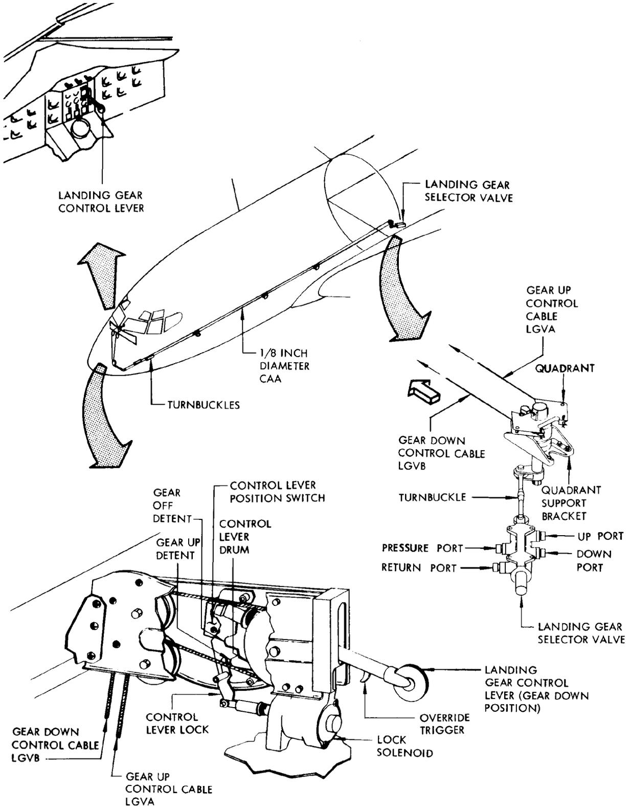
Landing Gear Control Components Location
