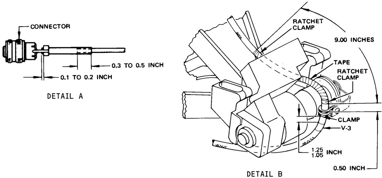
Main Gear Electrical Harness Installation
