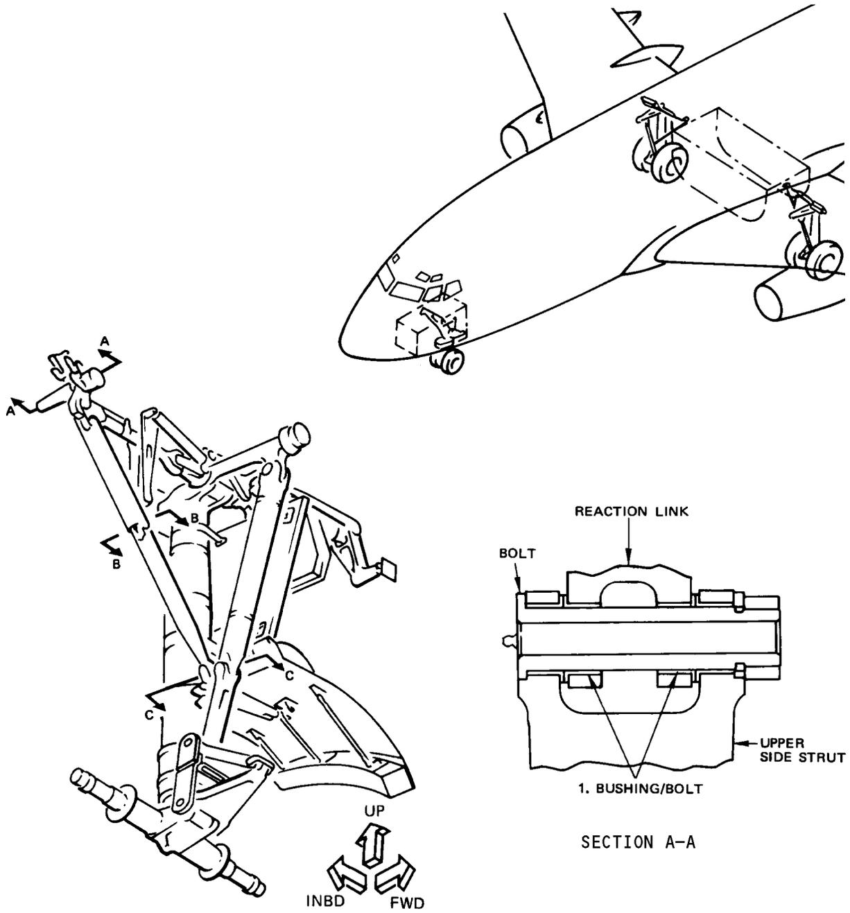
Main Gear Side Strut Wear Limits
