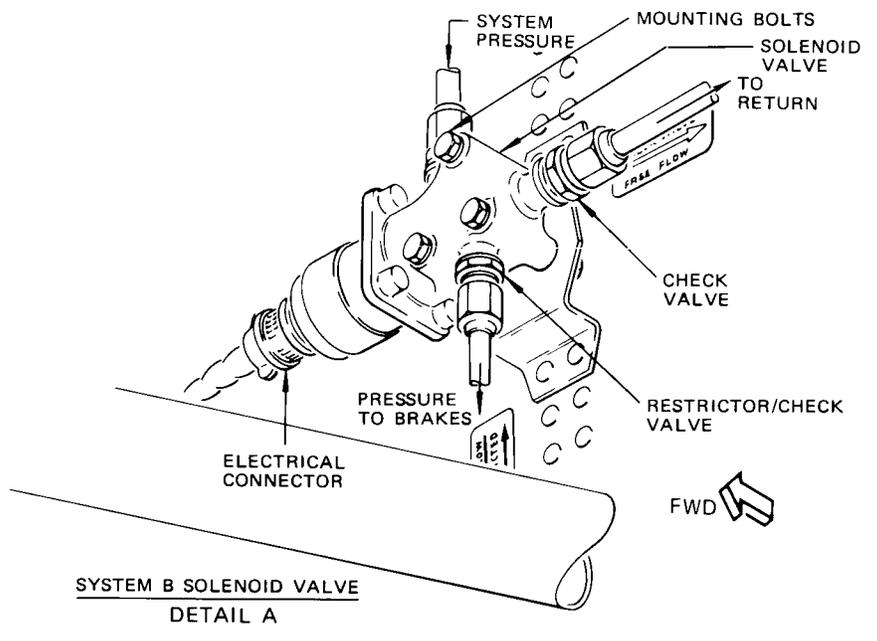
Autobrake Solenoid Valve Installation
