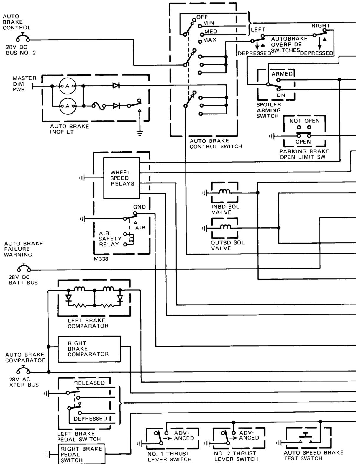
Automatic Braking System Control Circuit
