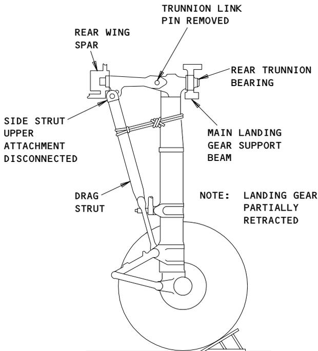
**STAGE 1. DISCONNECT DRAG STRUT AND REMOVE TRUNNION LINK PIN**
