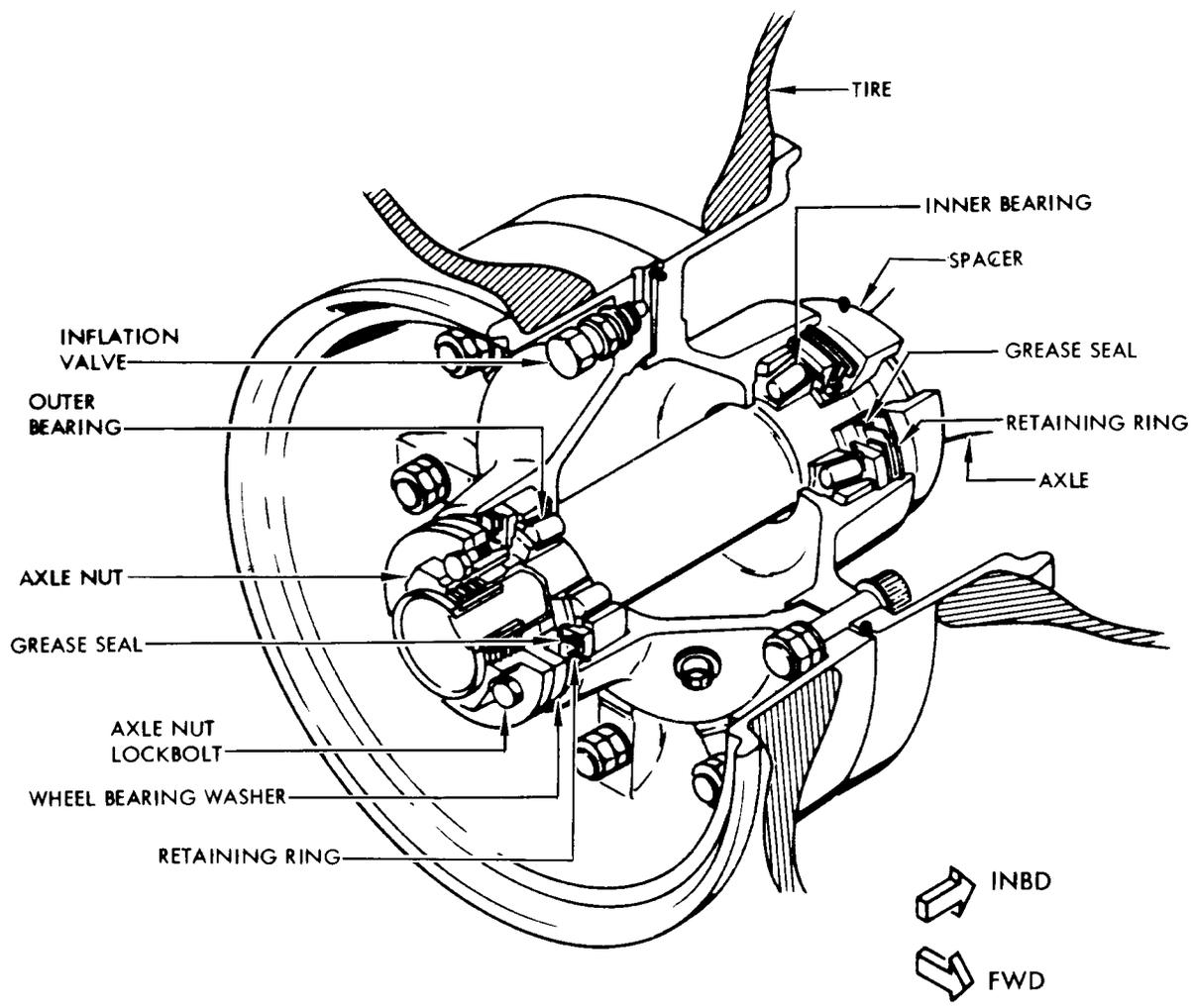
Nose Gear Wheel Installation
