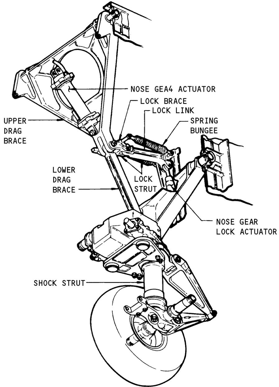
Nose Gear Extension and Retraction Components Location
