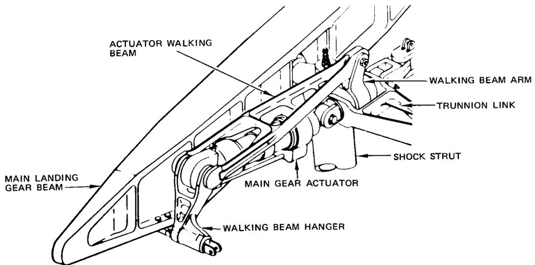
Actuator, Walking Beam and Beam Hanger Installation
