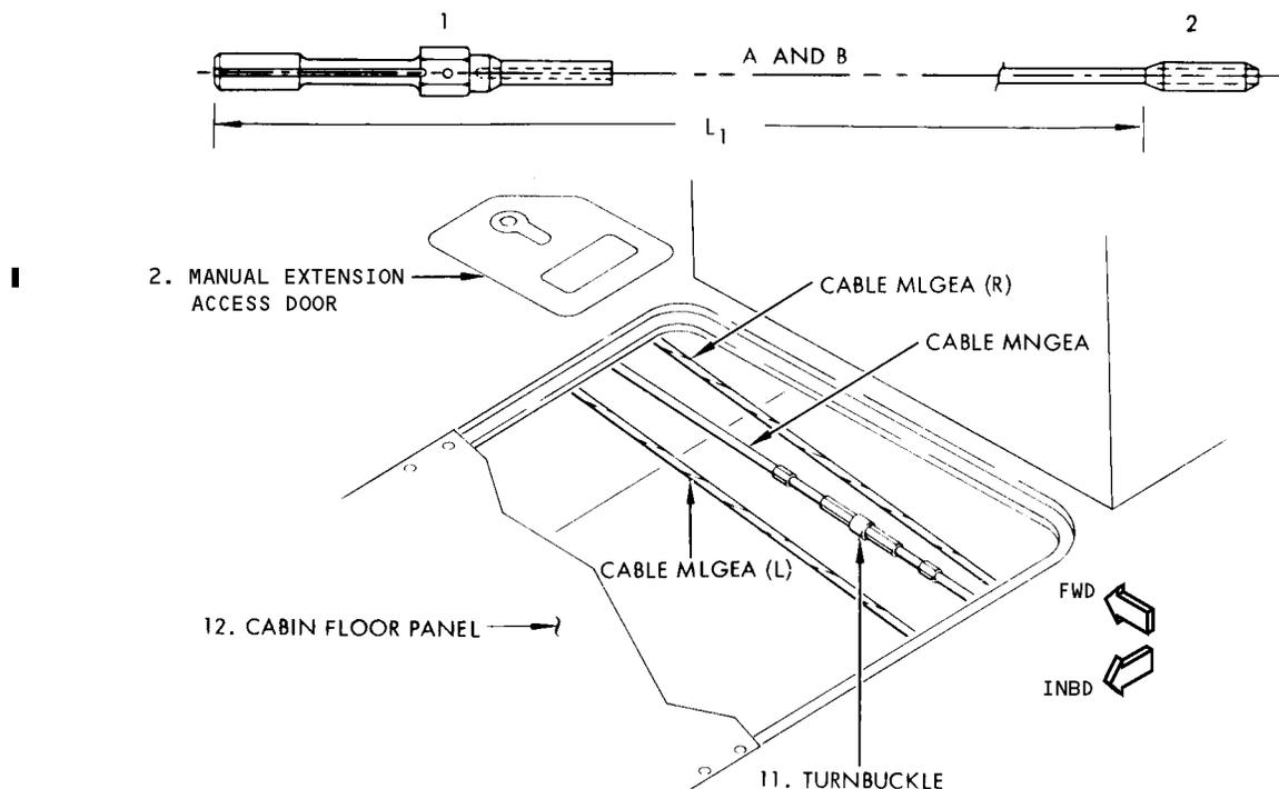
**Nose Gear Manual Extension System Cable Removal/Installation
