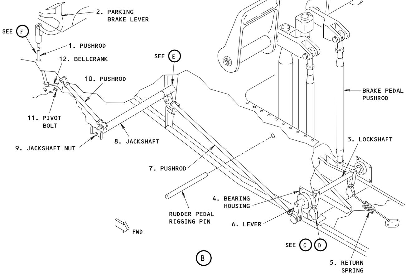
Parking Brake Linkage Installation
