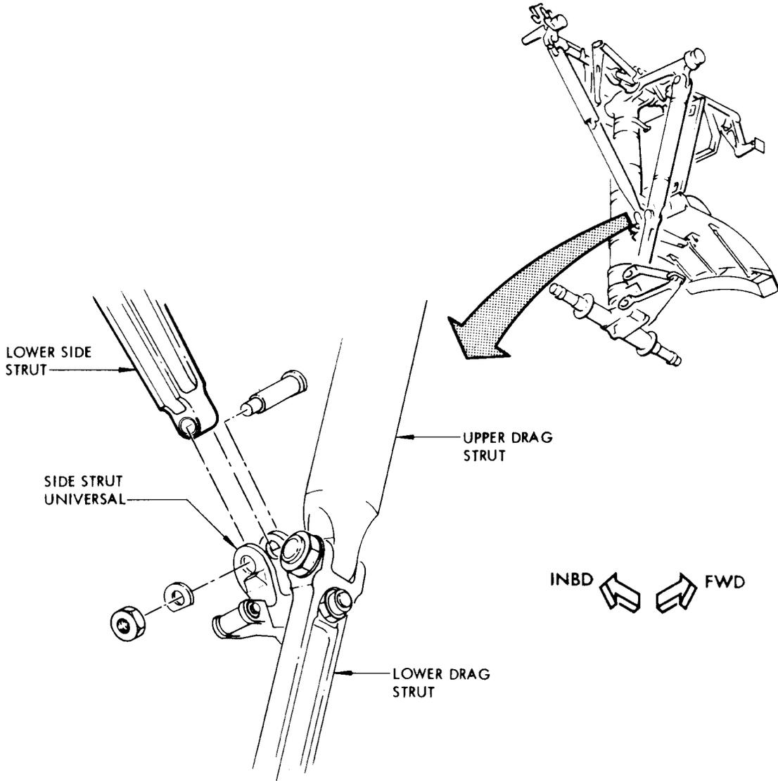
Main Gear Side Strut Lower Attachment
