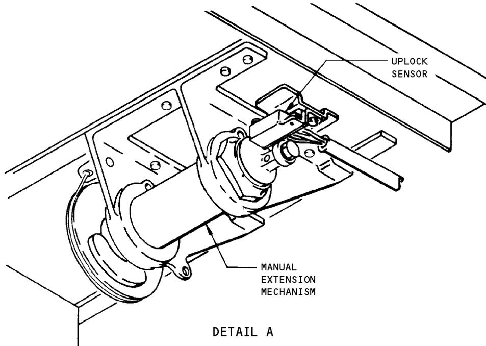
Nose Gear Uplock Sensor Installation
