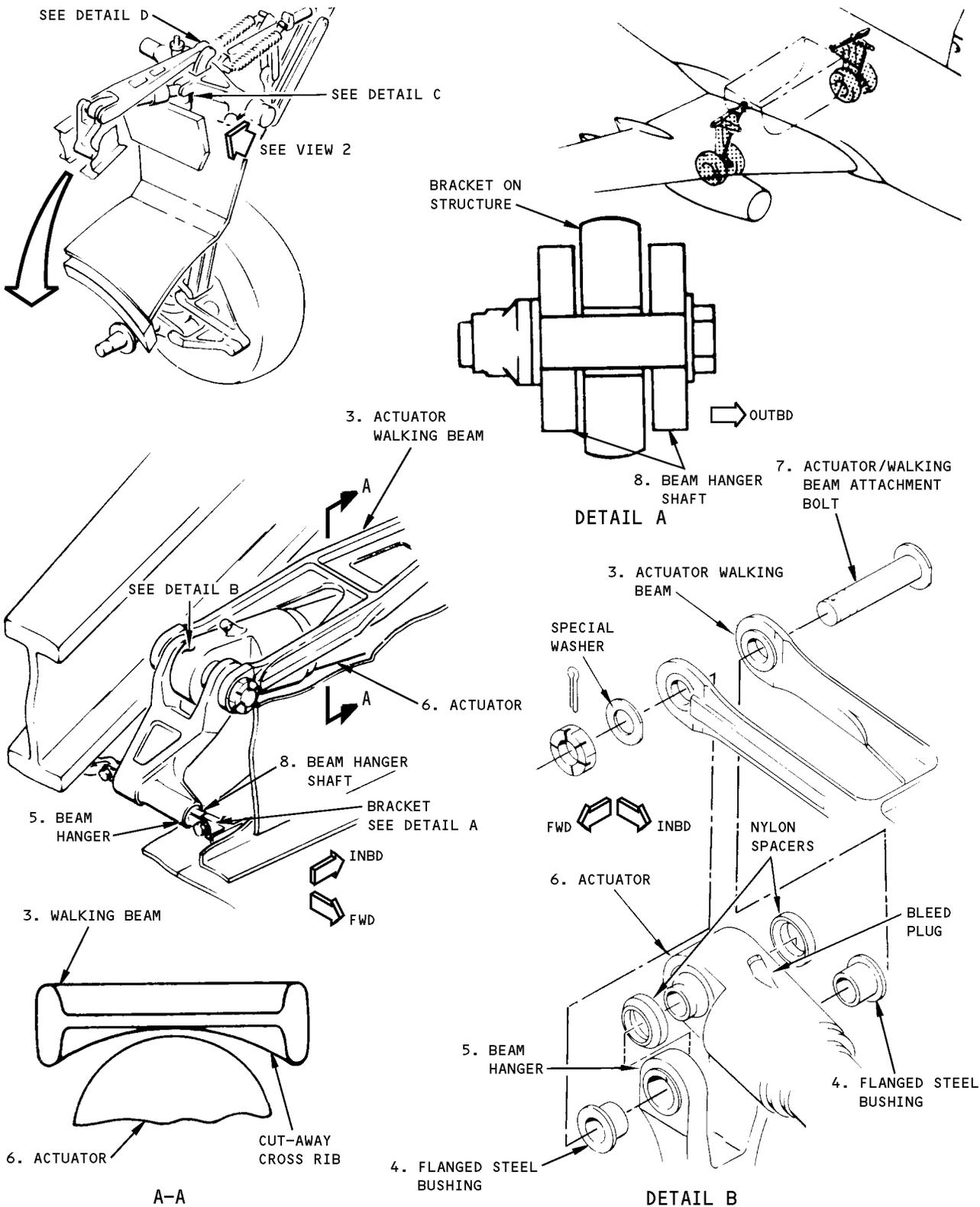
Main Gear Actuator Assembly Installation
