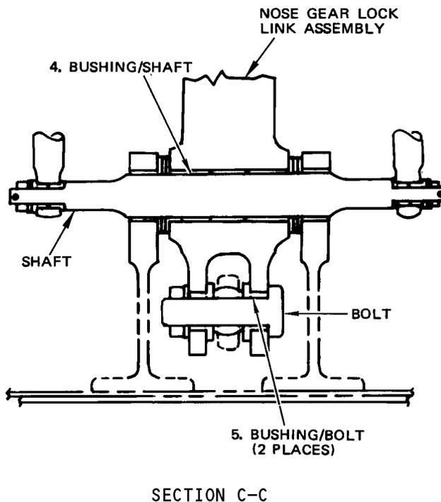
Nose Gear Lock Mechanism Wear Limits
