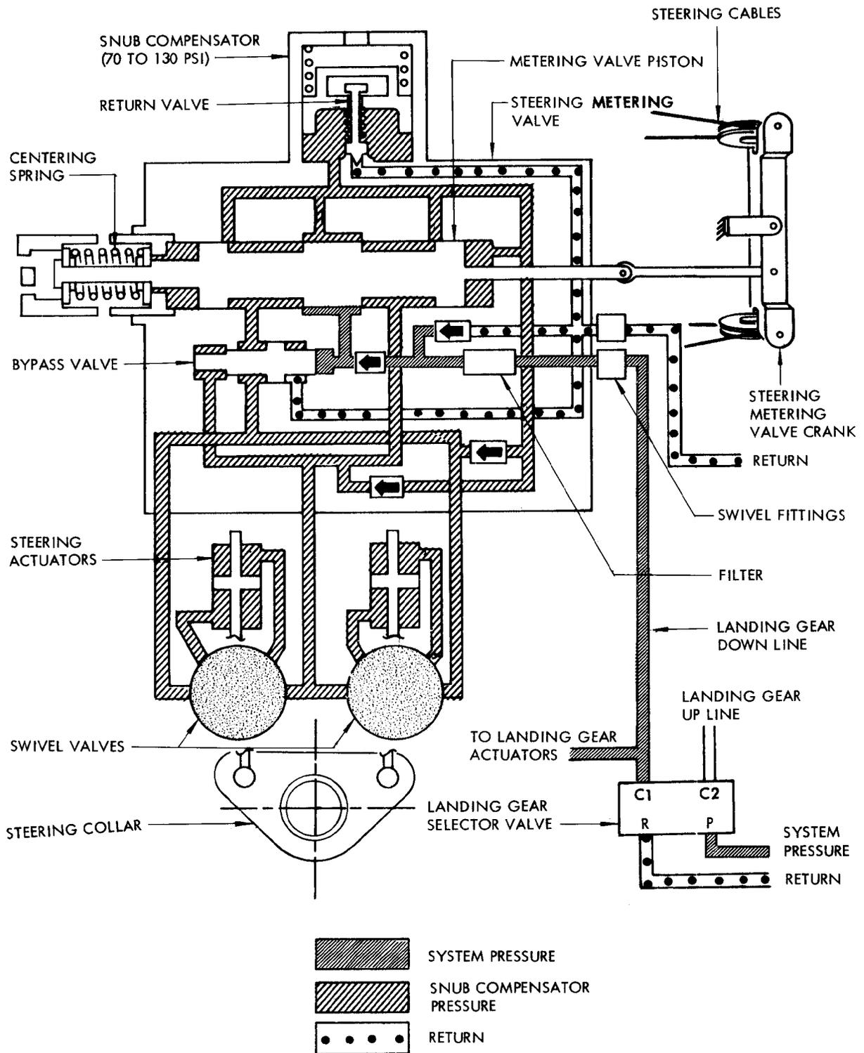
Nose Wheel Steering Schematic
