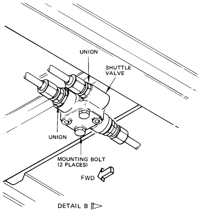
Autobrake Shuttle Valve Installation
