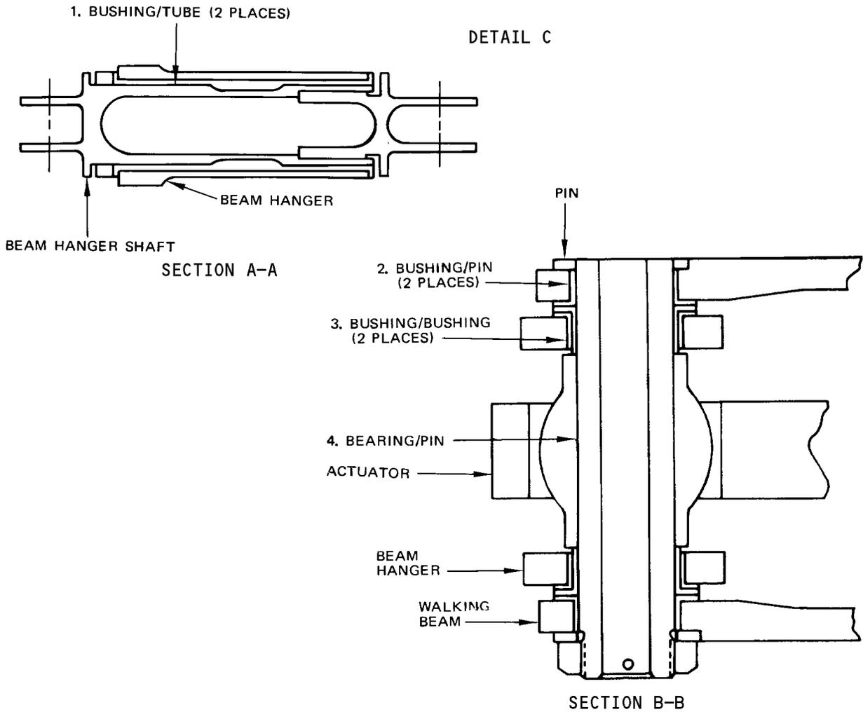
Main Gear Actuator Assembly Wear Limits
