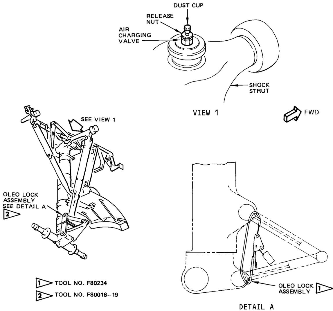
Shock Strut Air Charging Valve and Oleo Lock Assembly Installation
