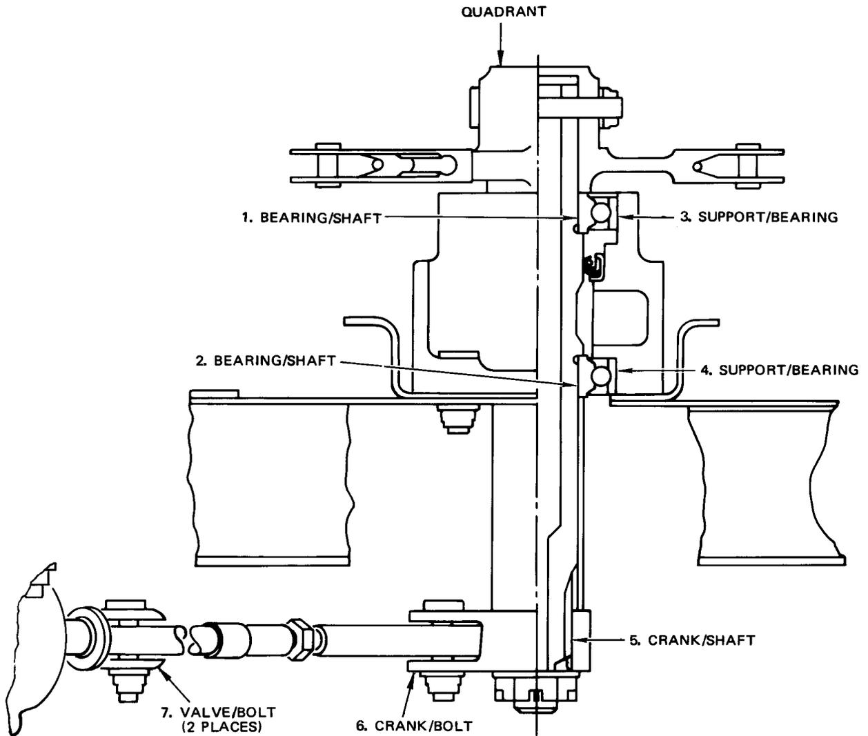
Landing Gear Selector Valve Control Quadrant Assembly Wear Limits
