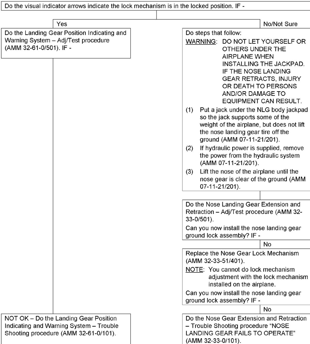
Testing and Fault Isolation
