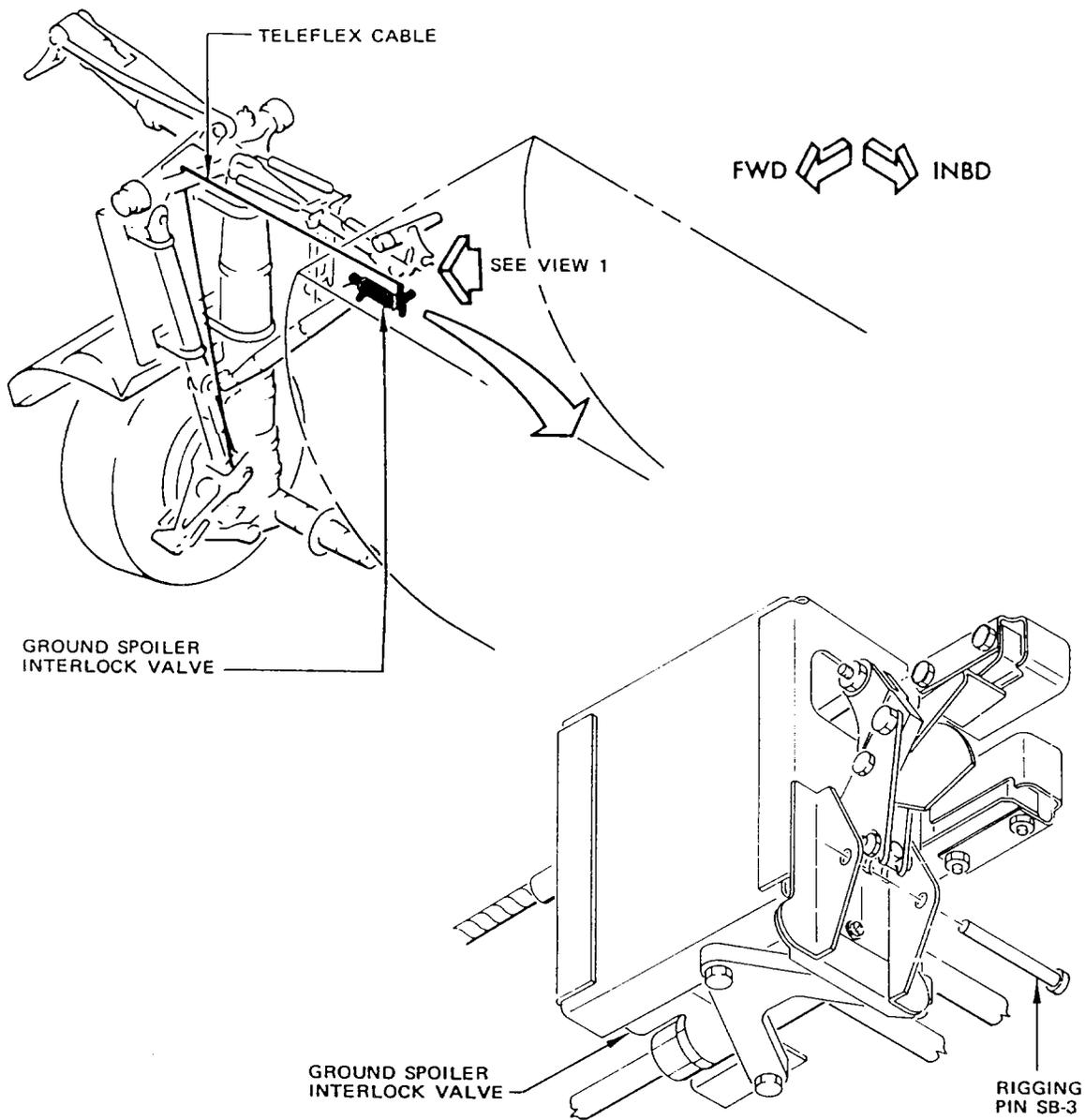
Landing Gear Safety Sensors Adjustment
