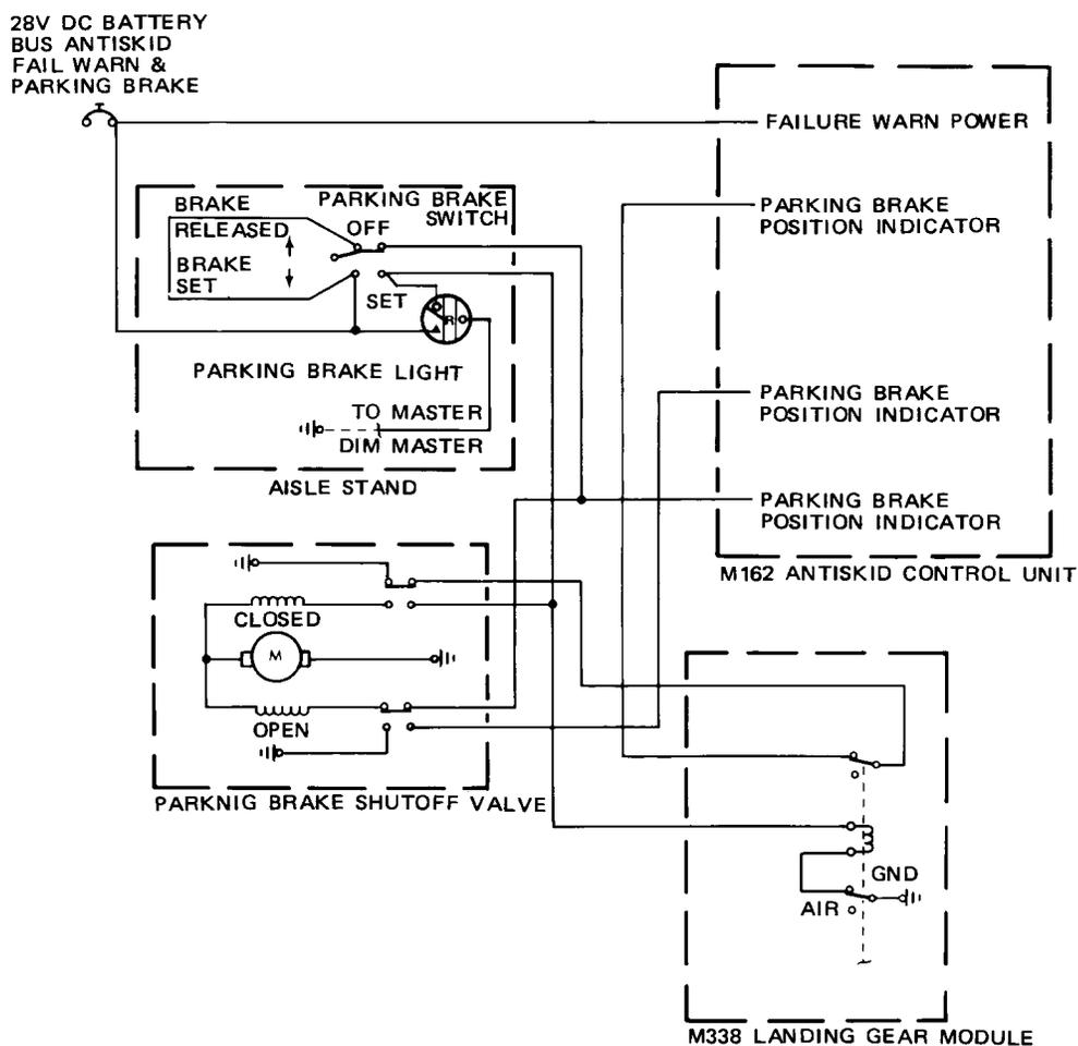
Parking Brake Shutoff Valve Circuit
