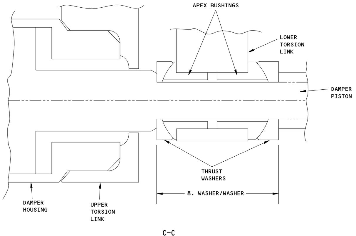
Main Gear Torsion Links Wear Limits
