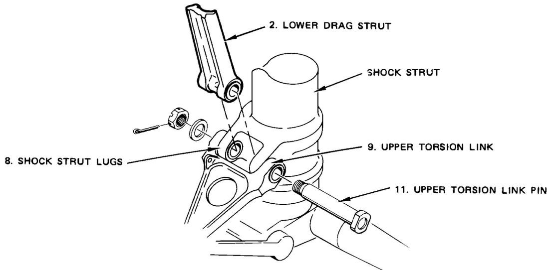
Main Gear Lower Drag Strut Installation
