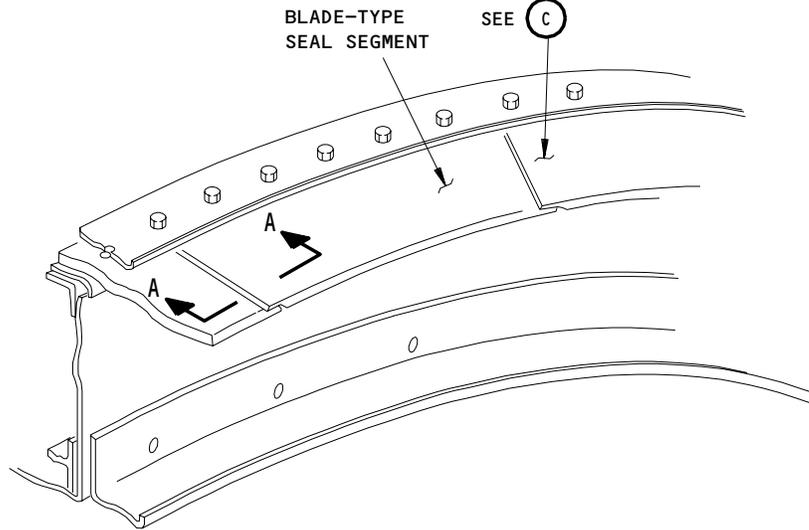
**BLADE-TYPE WHEEL WELL BLADE SEAL SEGMENT**
