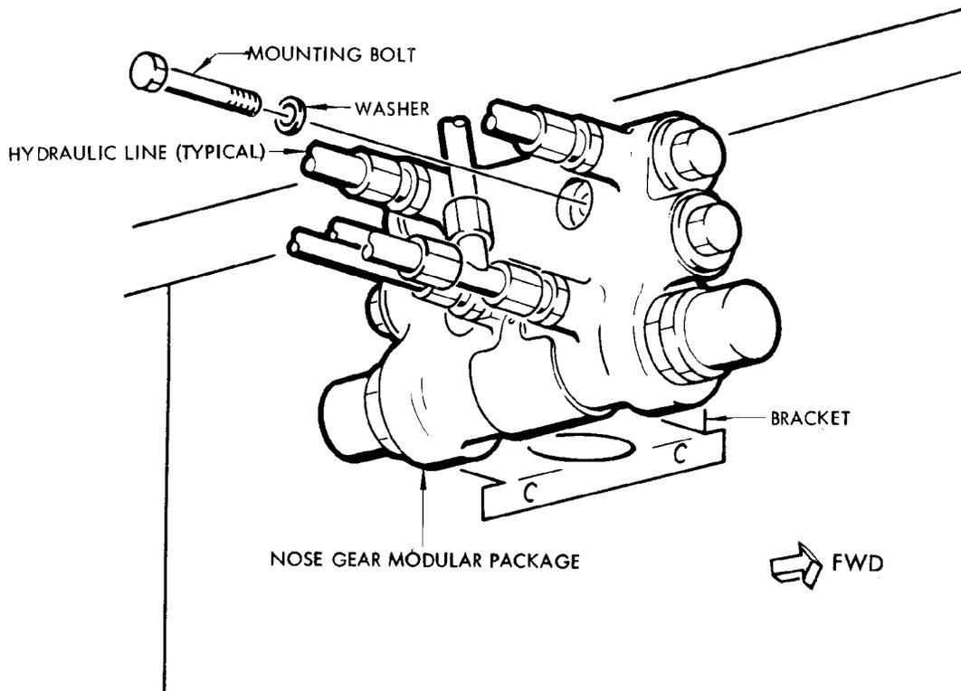
Nose Gear Modular Package Installation
