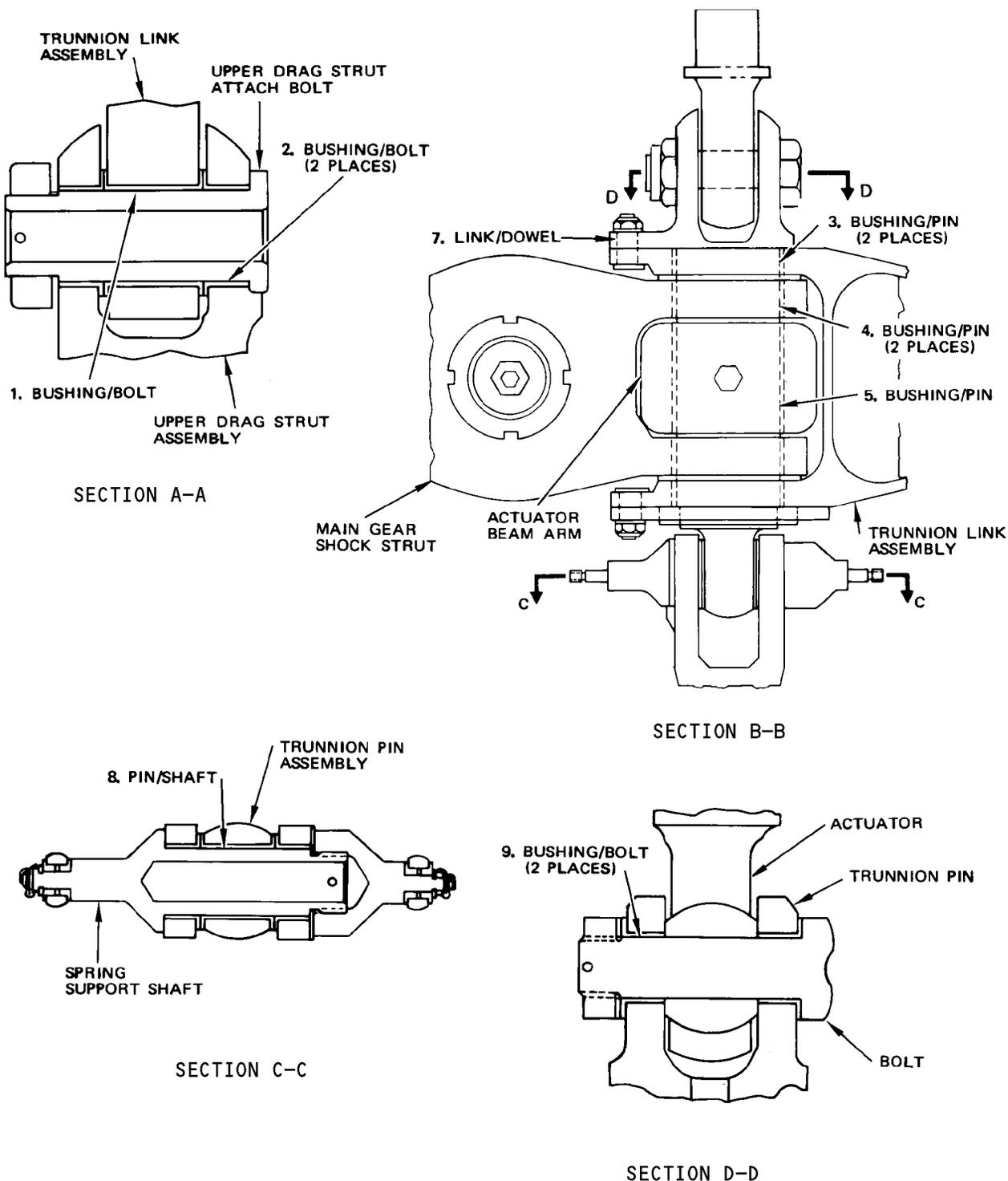
Main Gear Trunnion Link Assembly Wear Limits
