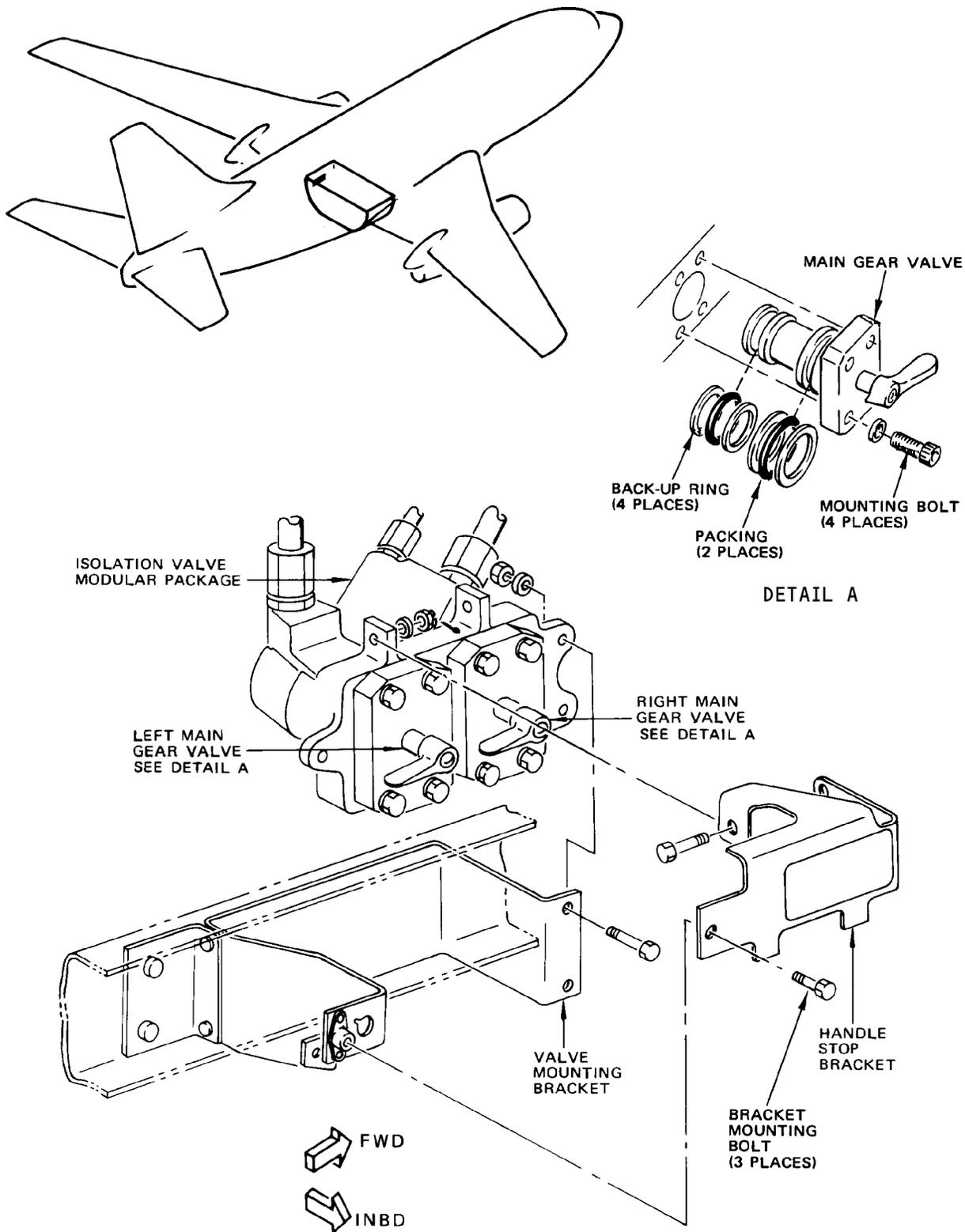
Main Gear Isolation Valves Installation
