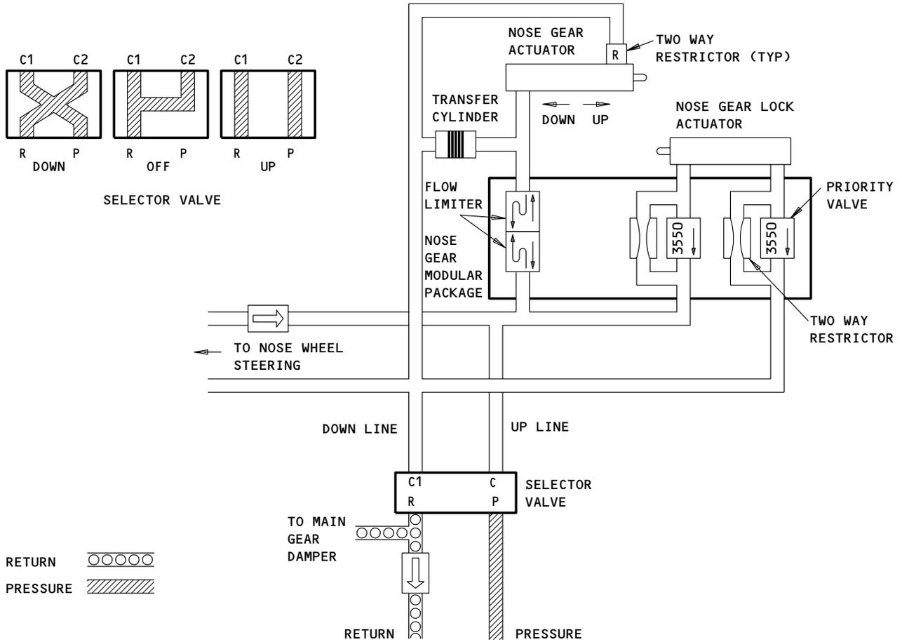
Nose Gear Hydraulic System Schematic
