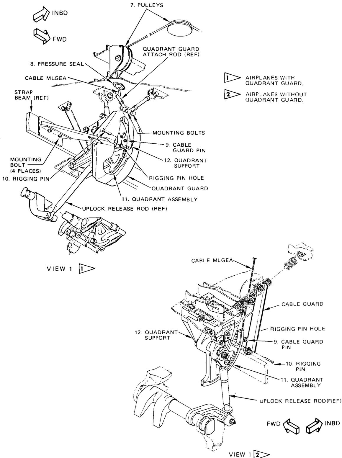
Main Gear Manual Extension System Cable Installation
