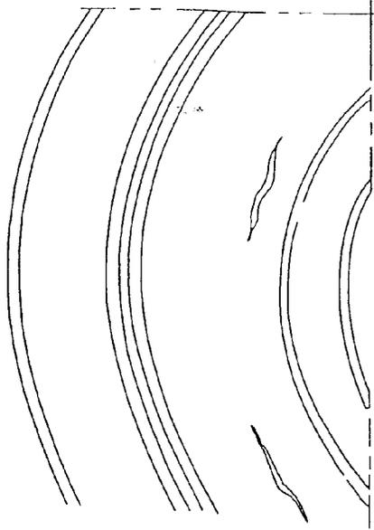
**Circumferential Sidewall Cracks**
