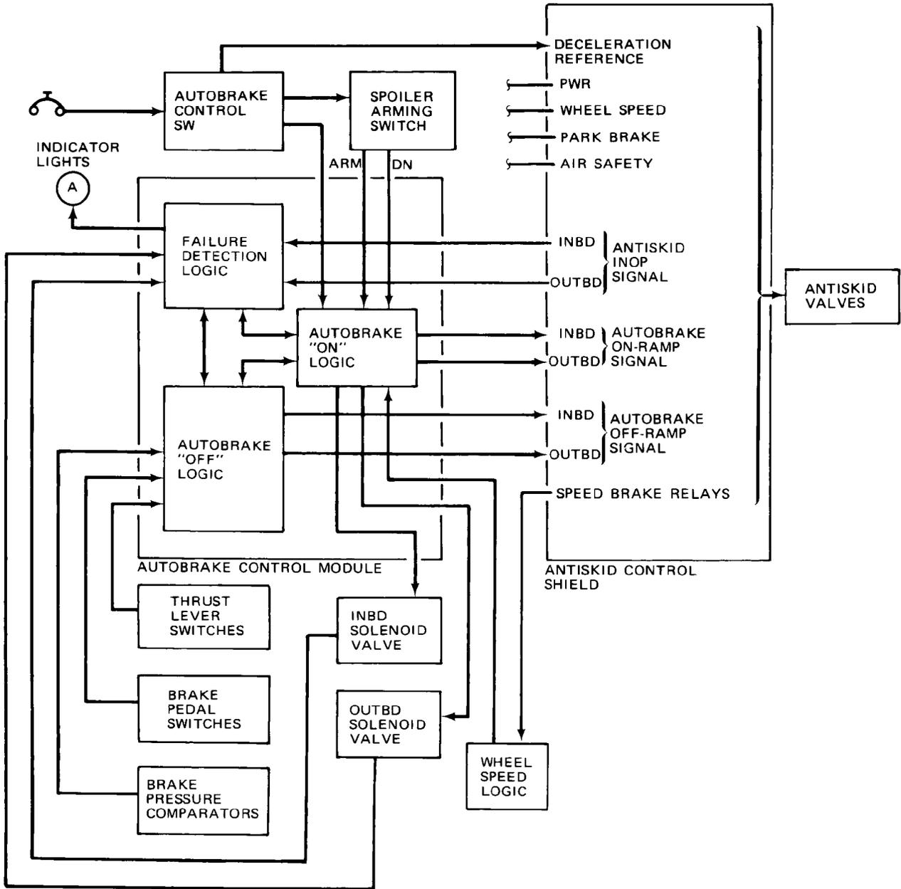
Automatic Braking System Block Diagram
