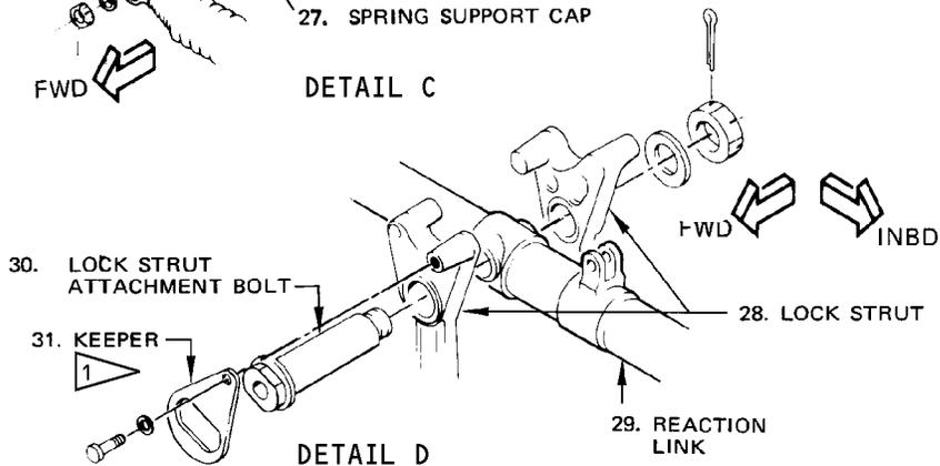
**Main Gear Trunnion Link Installation
