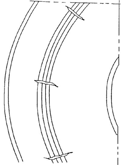
**Radial Sidewall Cracks**
