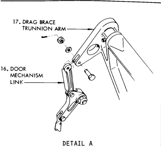
Nose Gear Drag Brace Installation
