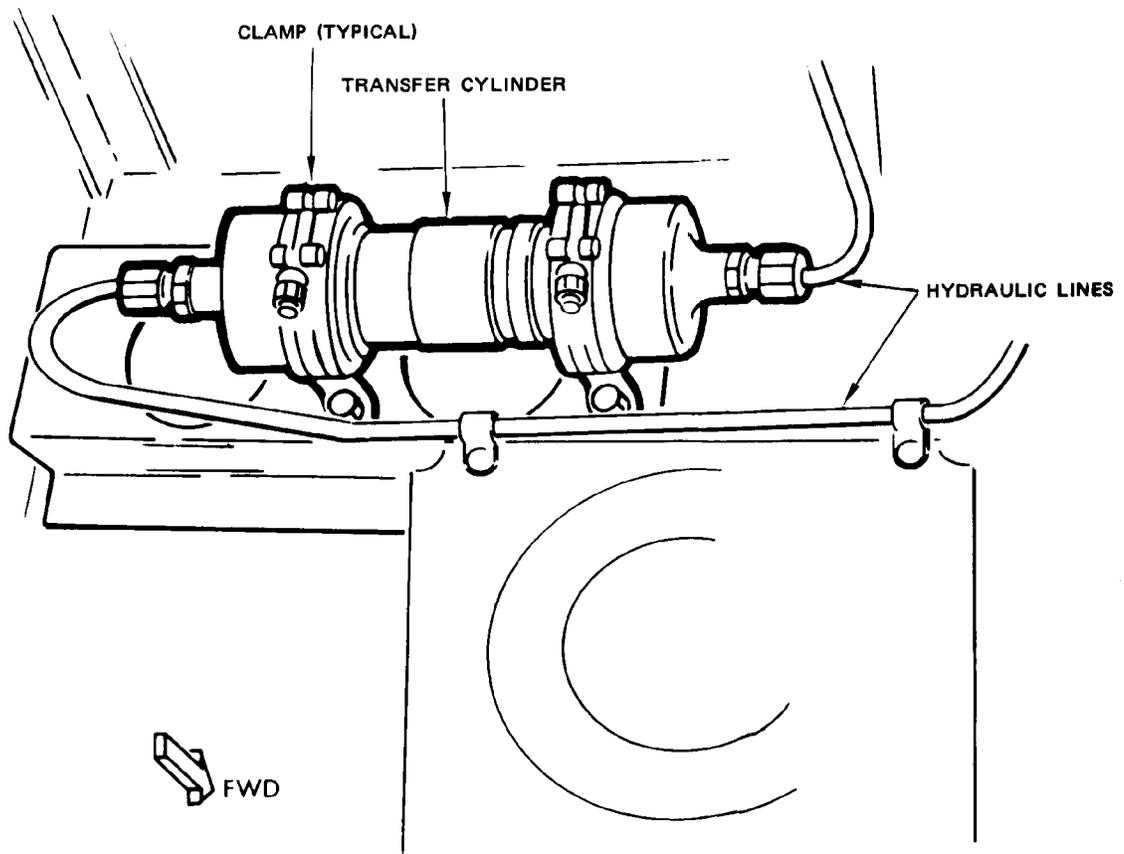
Nose Gear Transfer Cylinder Installation
