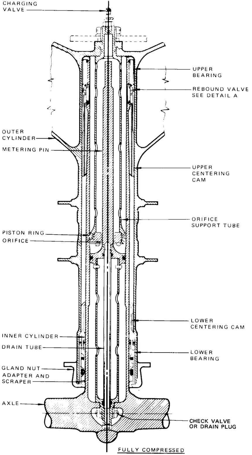
Nose Gear Shock Strut Schematic
