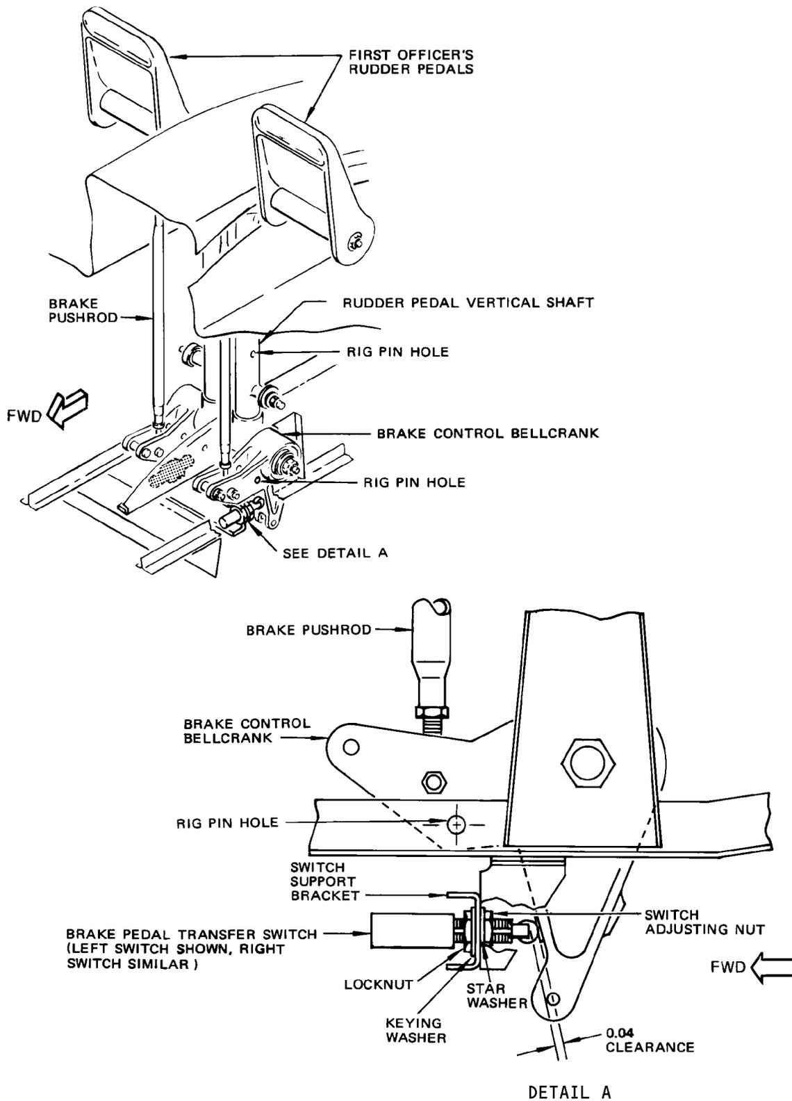
Brake Pedal Transfer Switch Installation
