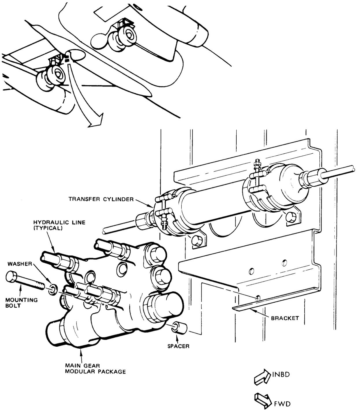
Main Gear Modular Package Installation
