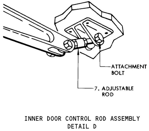
Main Gear Shock Strut Door Installation
