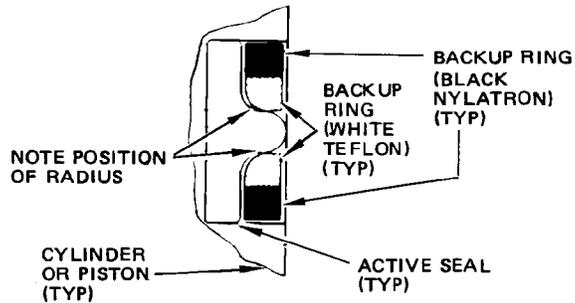
TYPICAL ACTIVE DYNAMIC SEAL ASSEMBLY INSTALLATION
