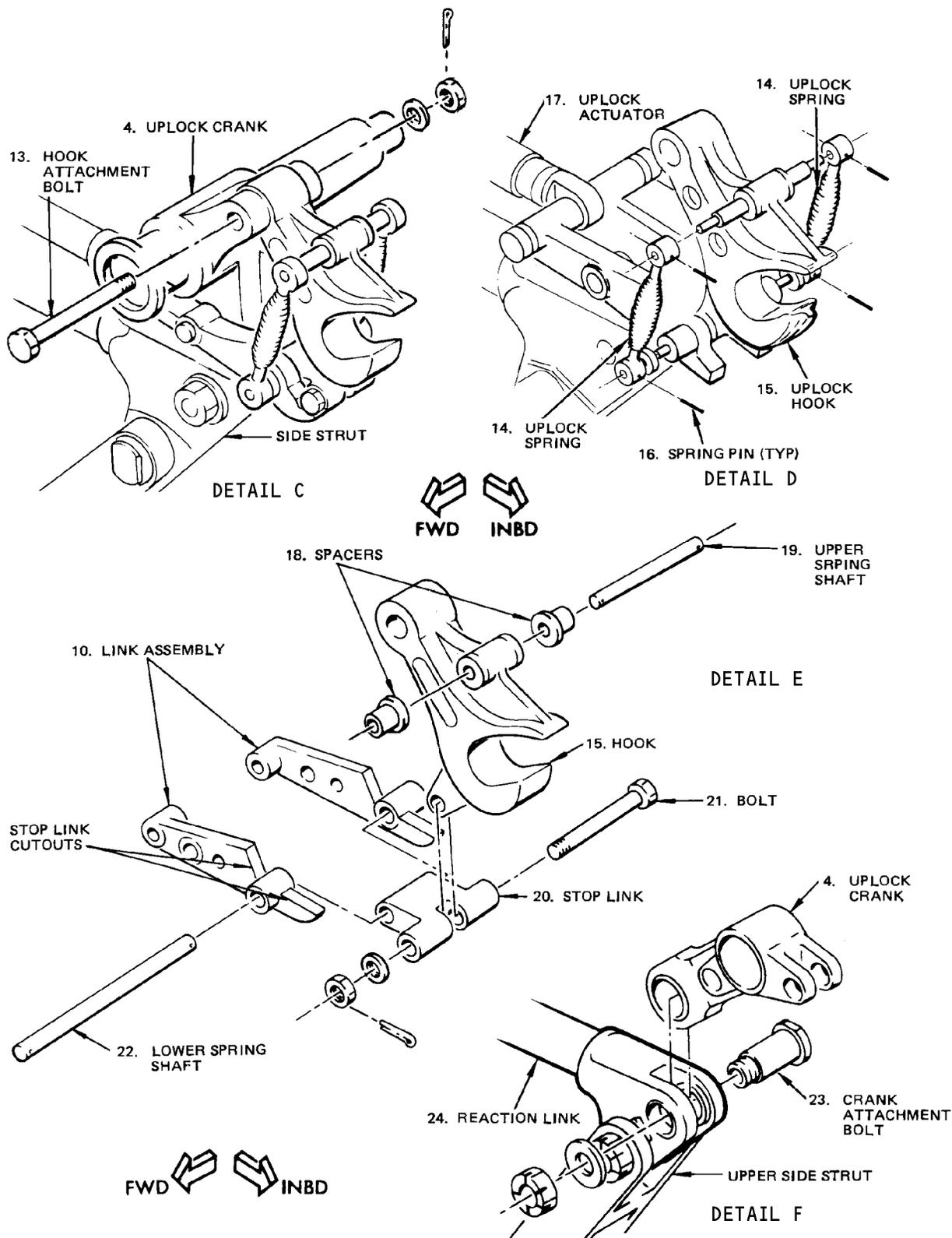
Main Gear Uplock Mechanism Installation
