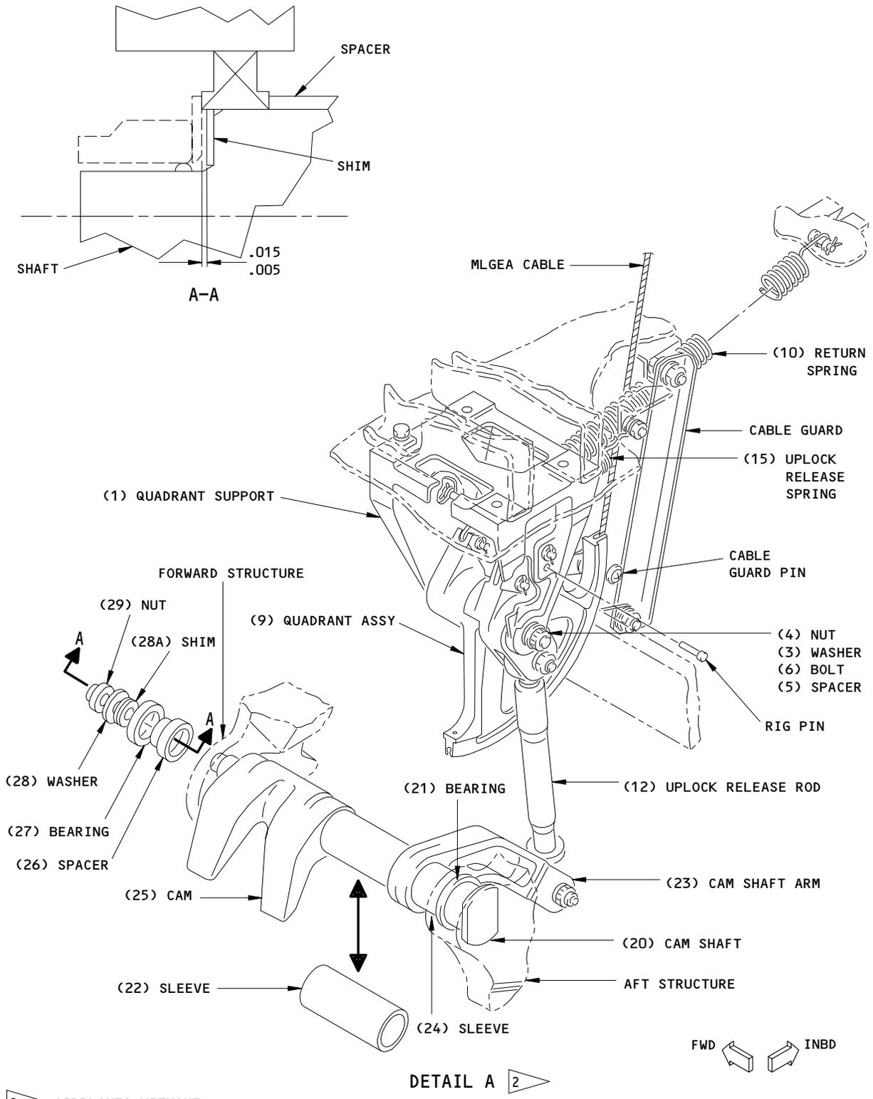
Main Gear Manual Extension Linkage Installation
