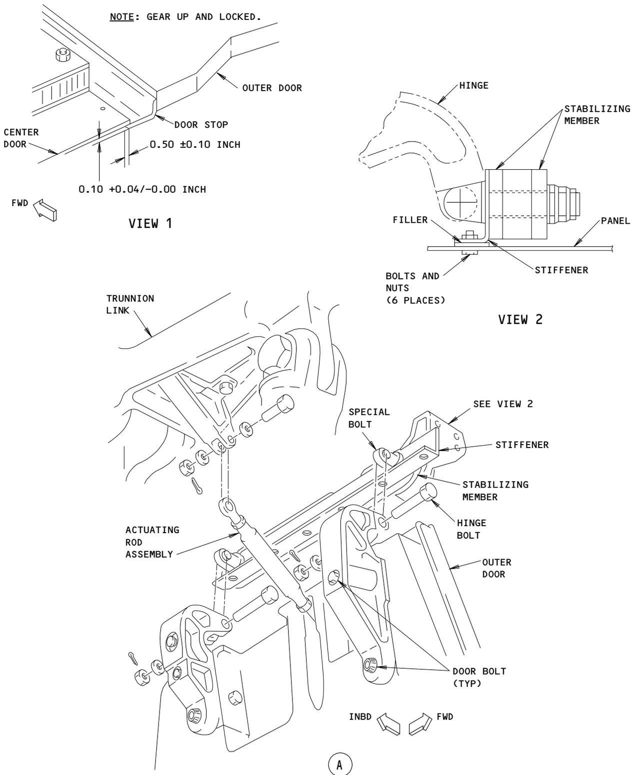
**Main Gear Wing Door Installation
