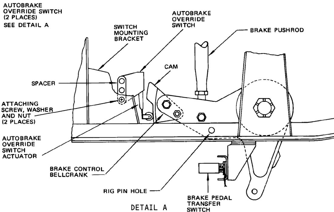
Autobrake Override Switch Installation
