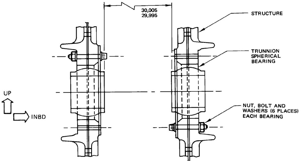
Nose Gear Trunnion Bearing Installation
