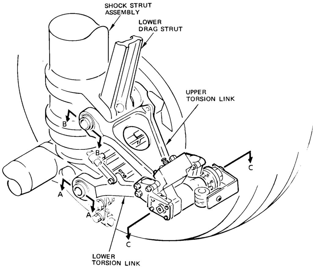
Main Gear Torsion Links Wear Limits
