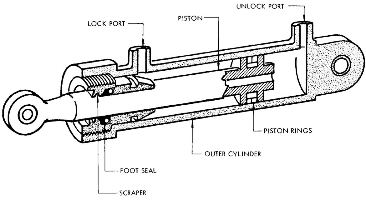
Main Gear Lock Actuator
