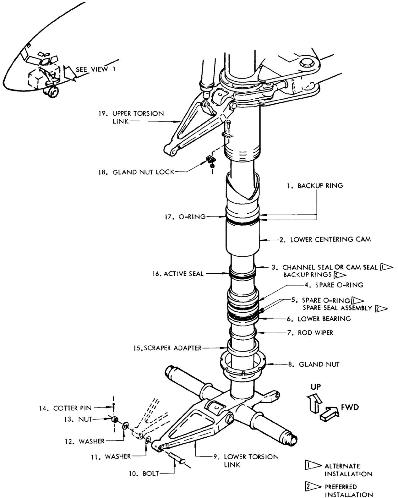
Nose Gear Shock Strut Seal Replacement
