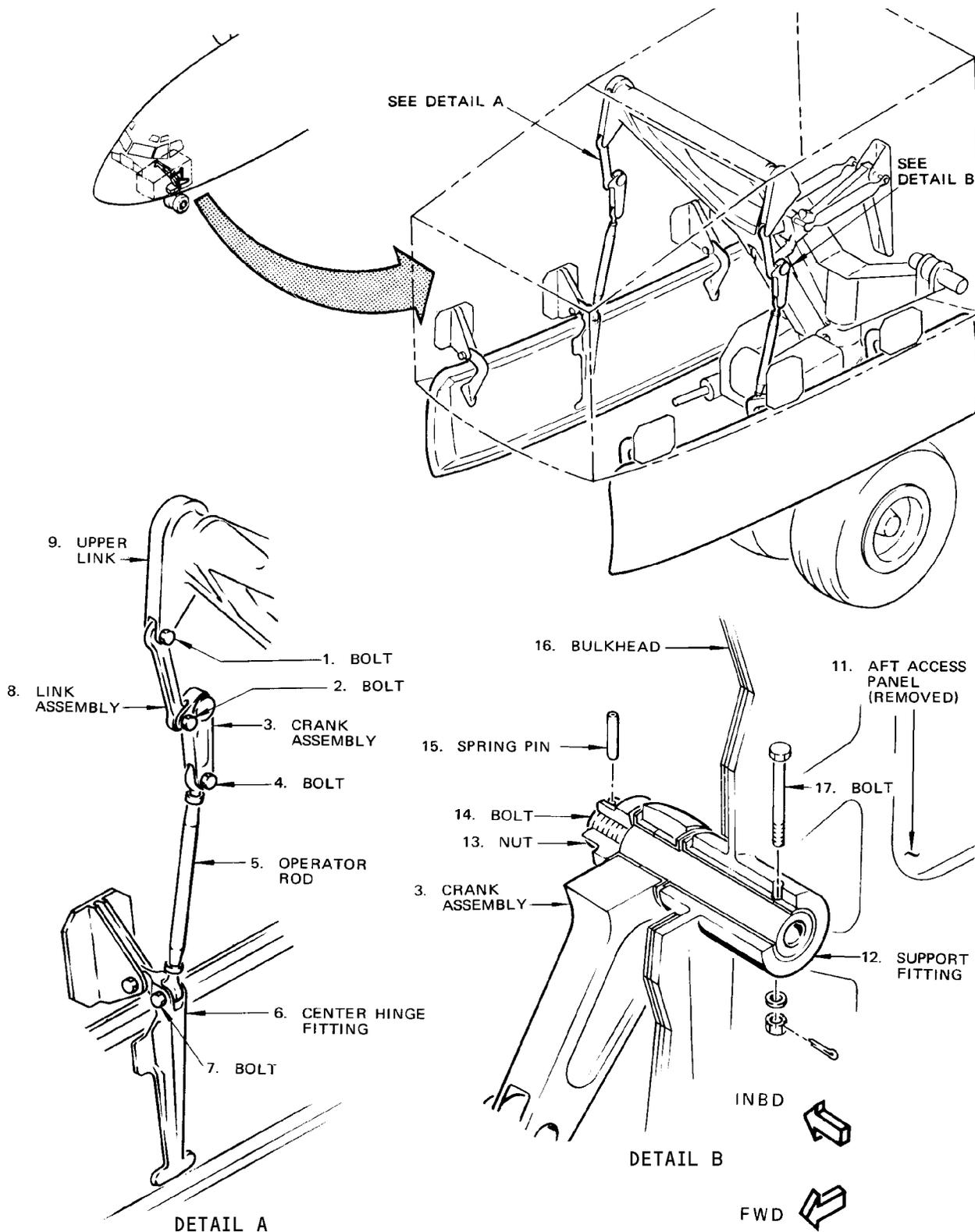
Nose Wheel Well Door Linkage Installation
