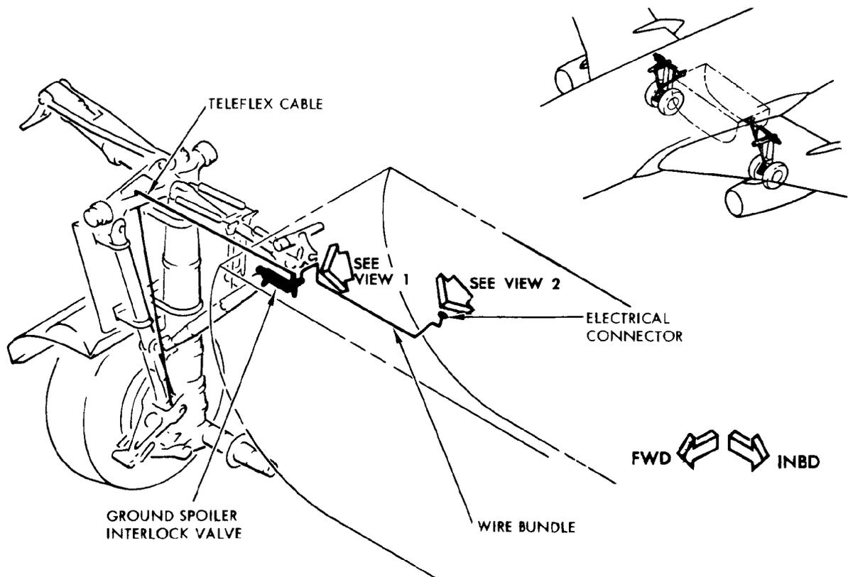
Landing Gear Safety Sensors Installation
