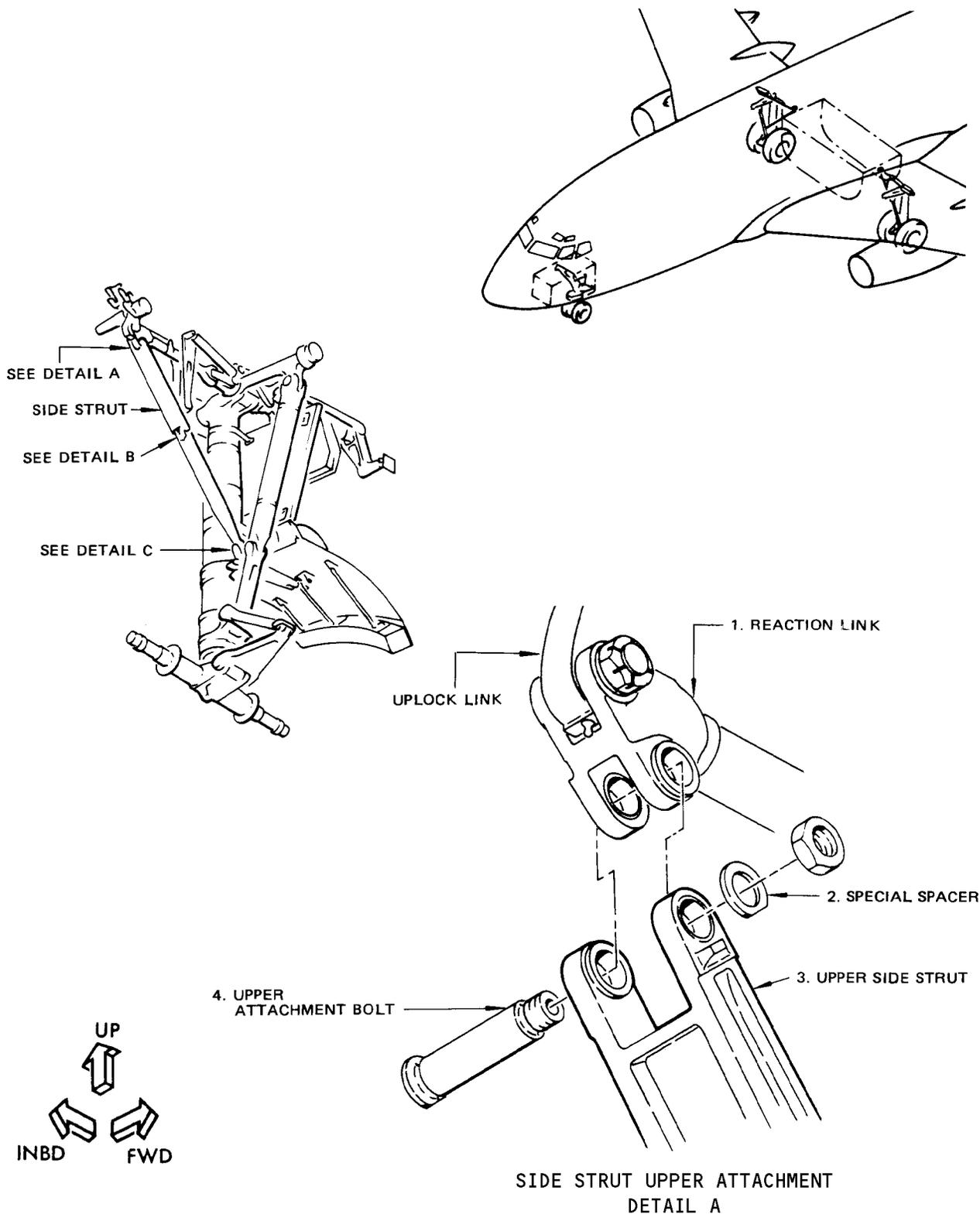
Main Gear Side Strut Installation
