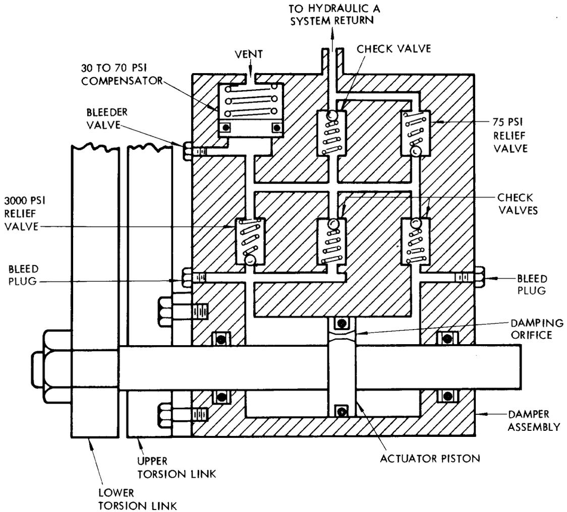
Main Landing Gear Damper Schematic
