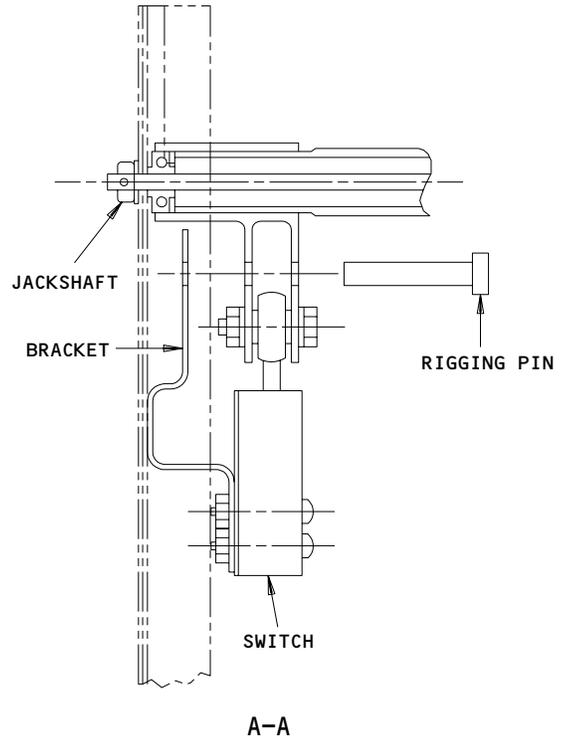
Parking Brake Linkage Adjustment
