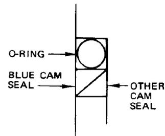
TYPICAL O-RING AND SPLIT CAM SEAL INSTALLATION
