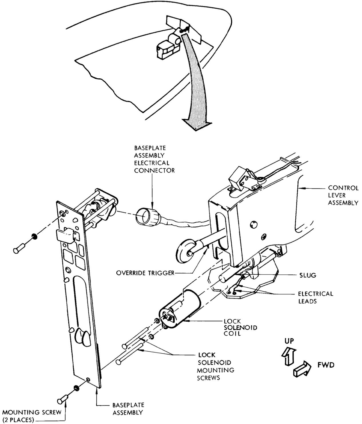
Landing Gear Control Lever Lock Solenoid Installation
