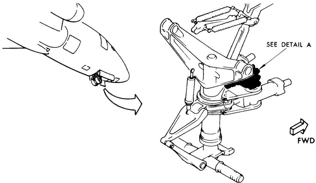
Steering Metering Valve Installation
