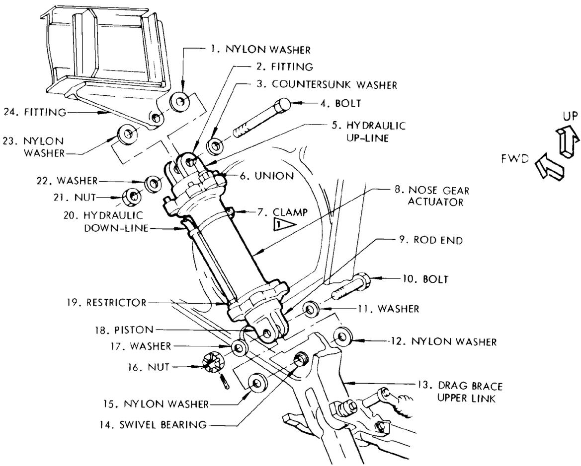
Nose Gear Actuator Installation
