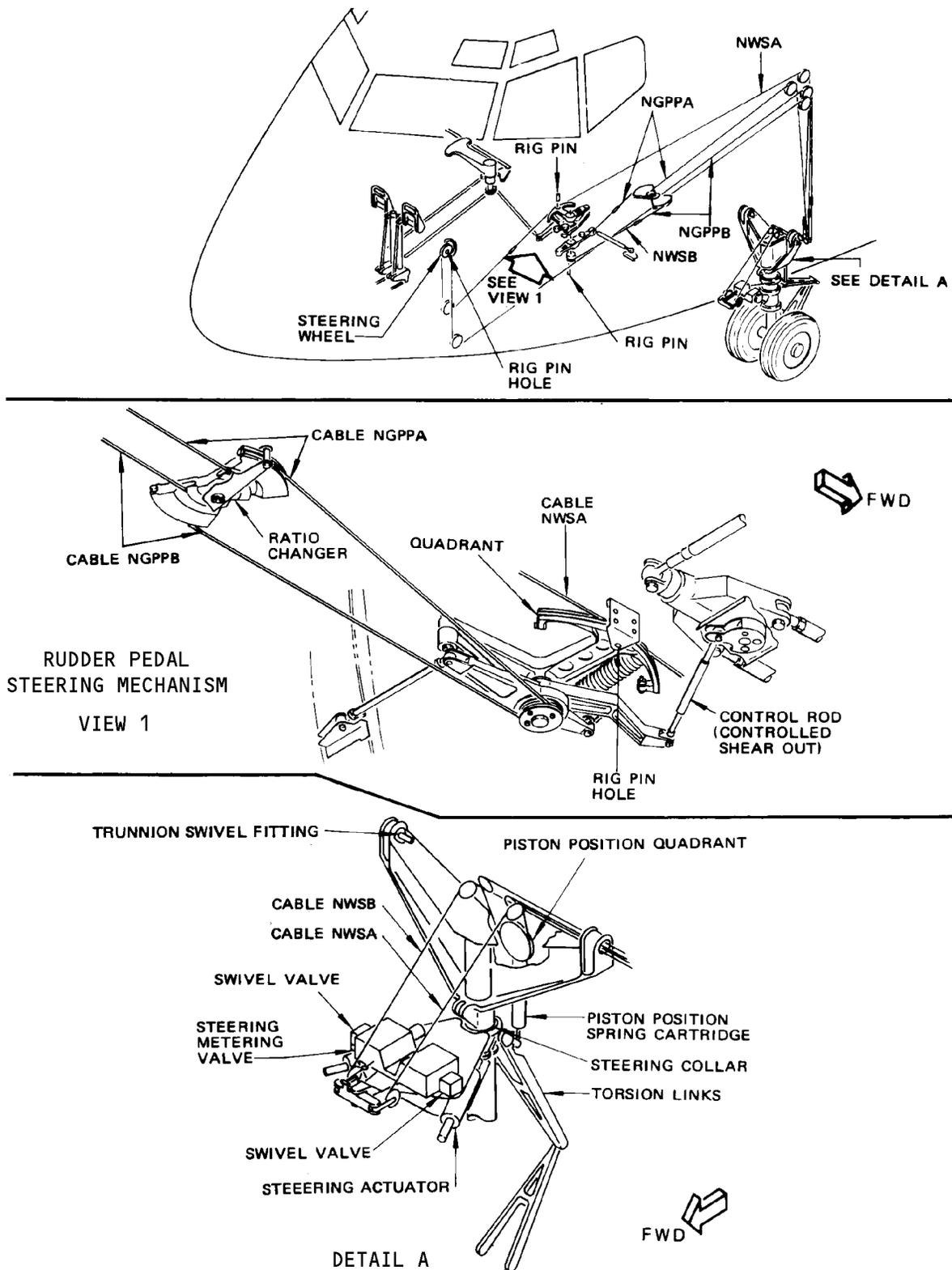
Nose Wheel Steering System Component Location
