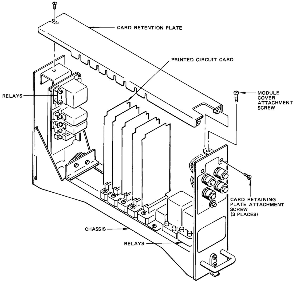
NOTE: CONTROL MODULE COVER SHOWN REMOVED
