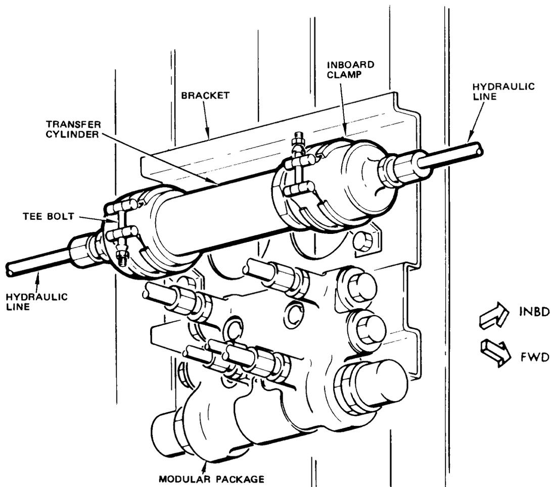
Main Gear Transfer Cylinder Installation
