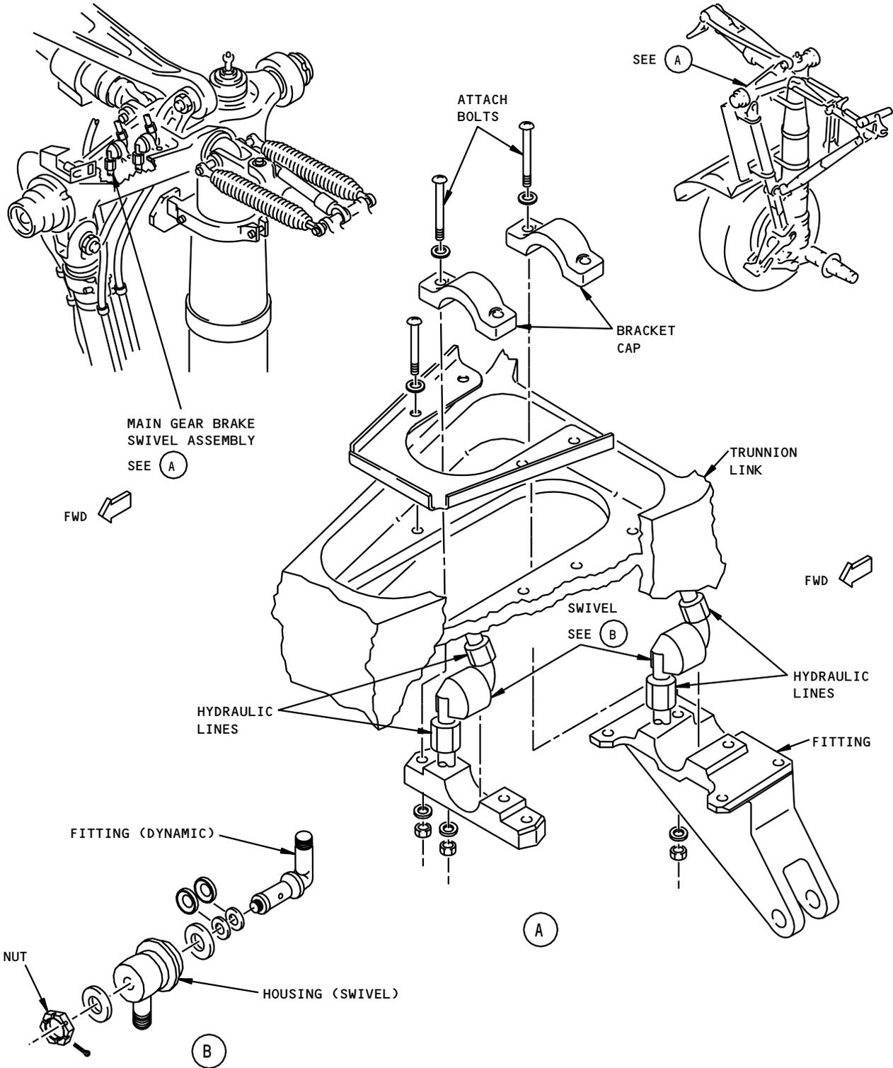
Main Gear Brake Swivel Installation
