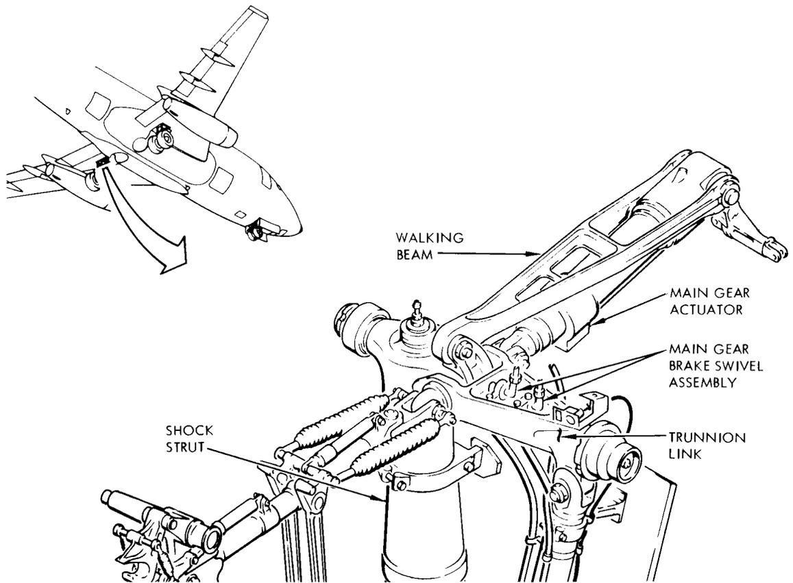
Main Gear Brake Swivel Assembly
