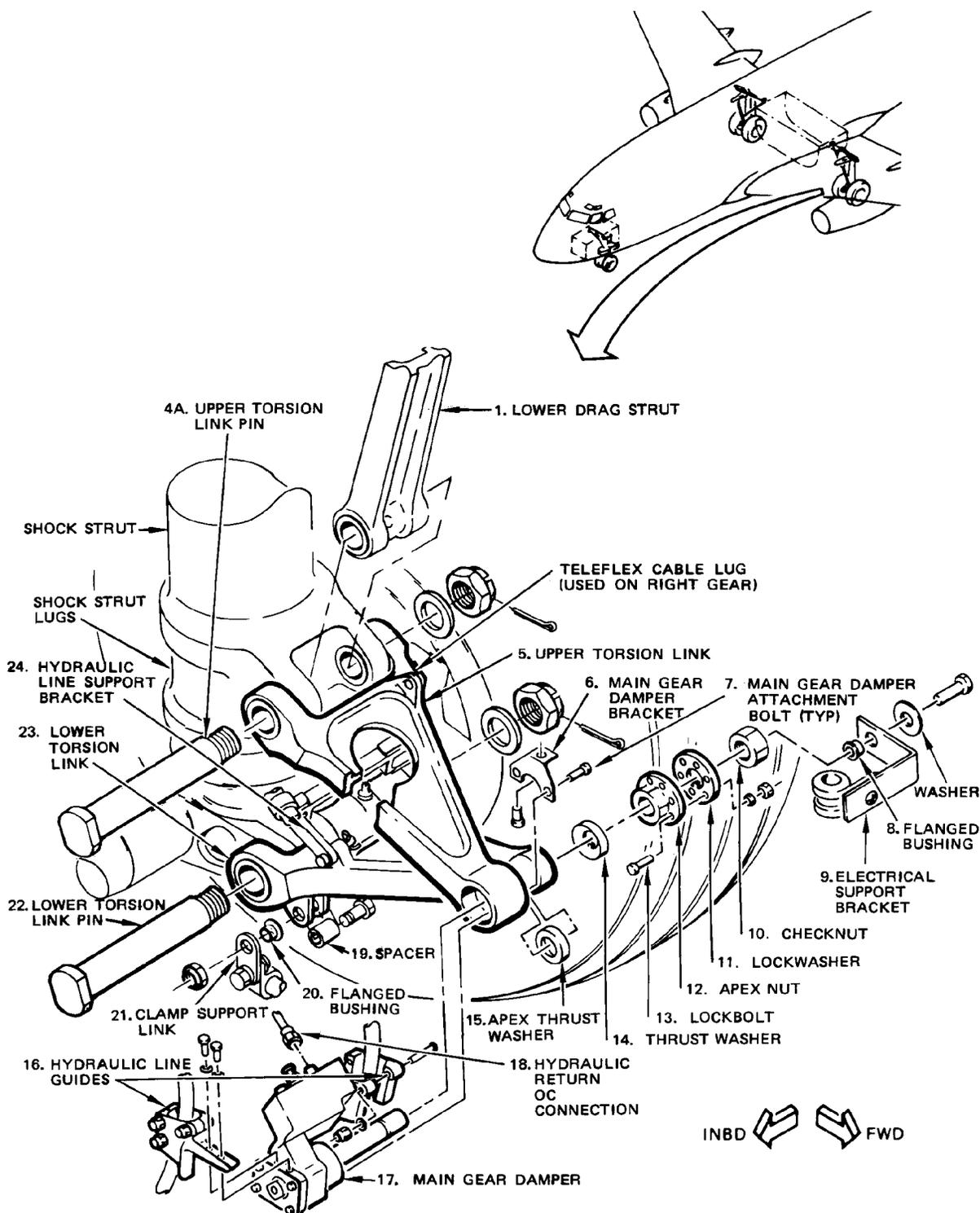
Left Main Gear Torsion Links Attachment
