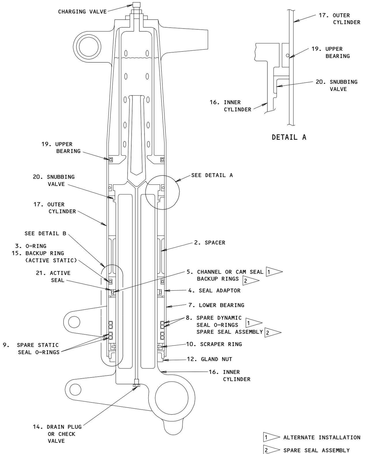
**Main Gear Shock Strut Seal Replacement
