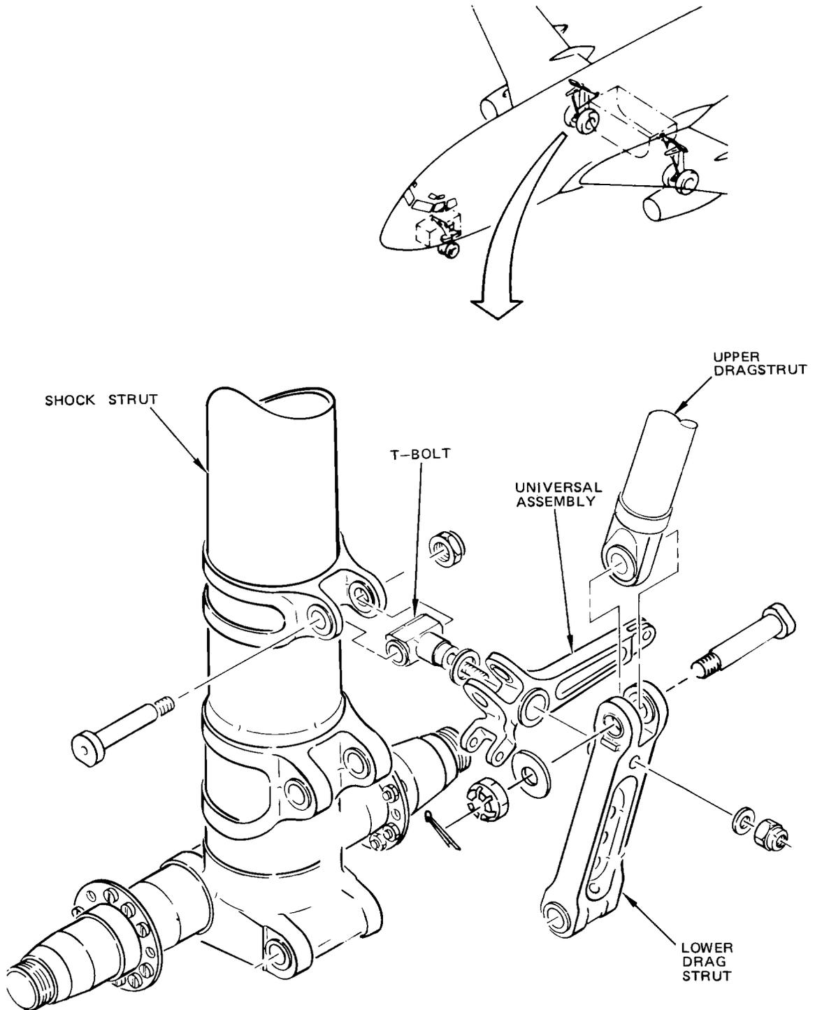
Main Gear T-Bolt Installation
