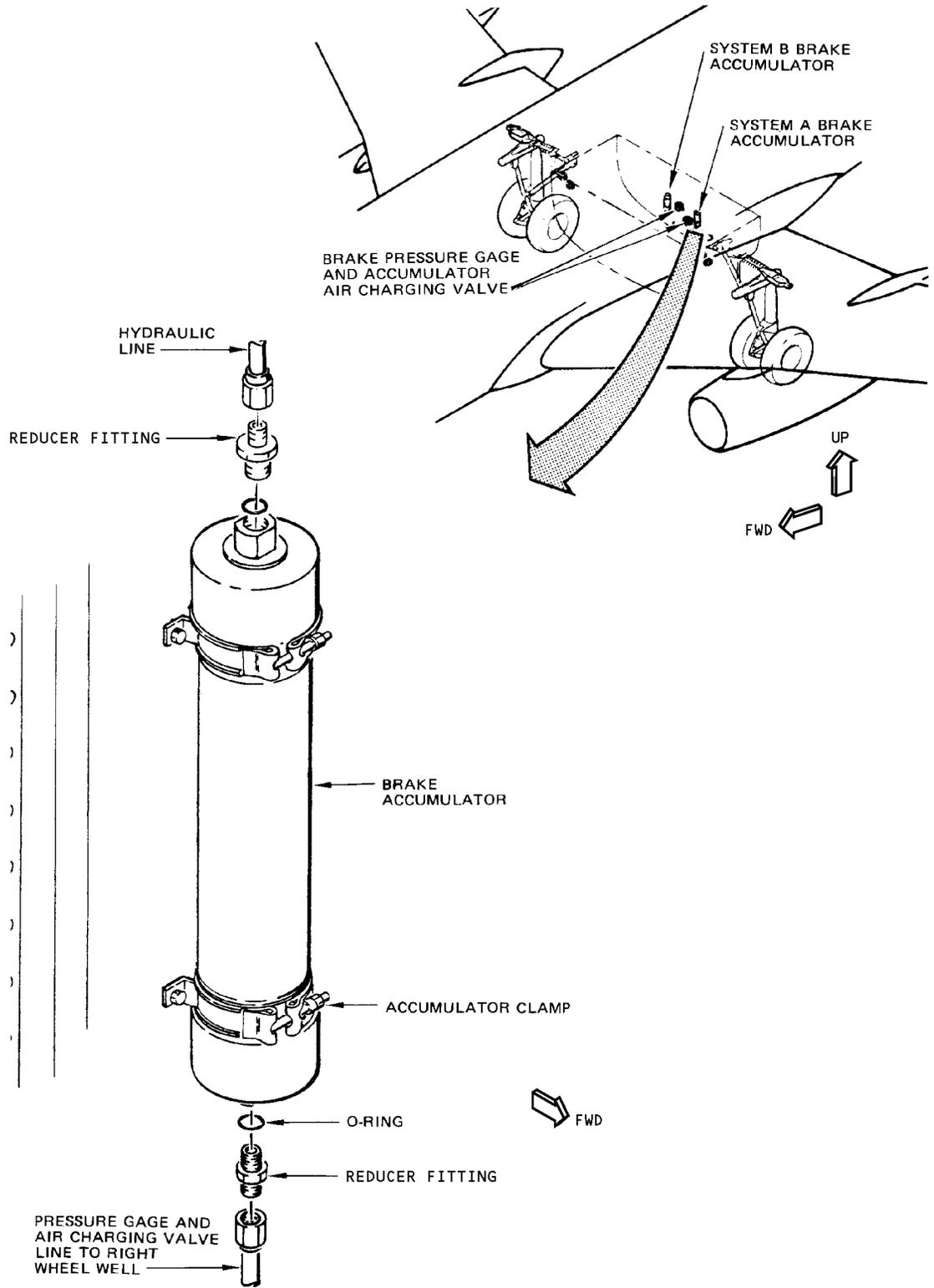
Brake Accumulator Installation
