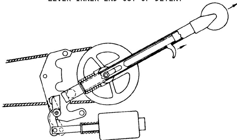
OVERRIDE TRIGGER PULLED TO ALLOW INNER END OF LEVER TO CLEAR LOCK STOP
