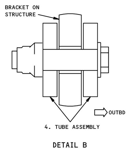
Main Gear Beam Hanger Shaft Installation
