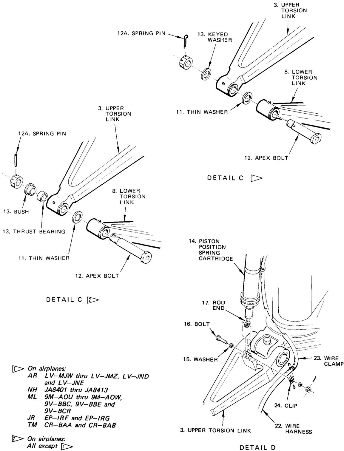
Nose Gear Torsion Link Installation
