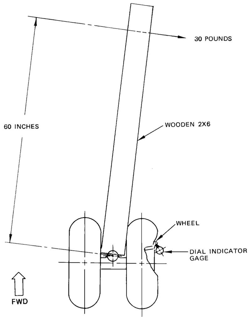
Nose Landing Gear Torsional Free Play Inspection
