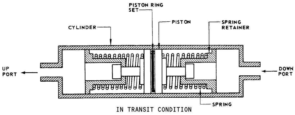
Transfer Cylinder Schematic
