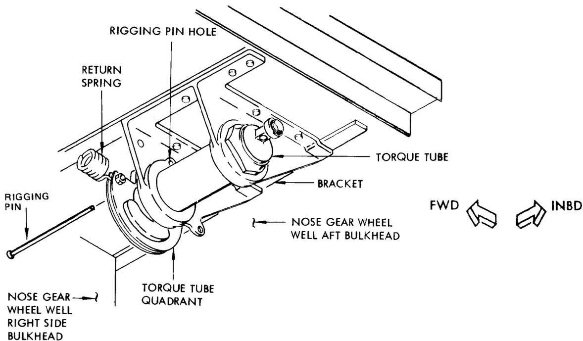
TORQUE TUBE AND BRACKET ASSEMBLY
