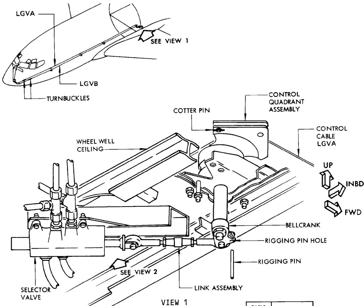
▶ AFTER INITIAL RIGGING, ANY DEVIATION OF  $\pm 15$  POUNDS AT 22°F OR ABOVE SHALL REQUIRE THAT THE SYSTEM BE RERIGGED.
