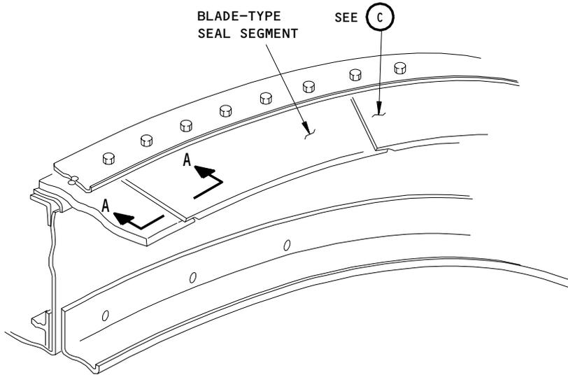
**BLADE-TYPE WHEEL WELL BLADE SEAL SEGMENT**
