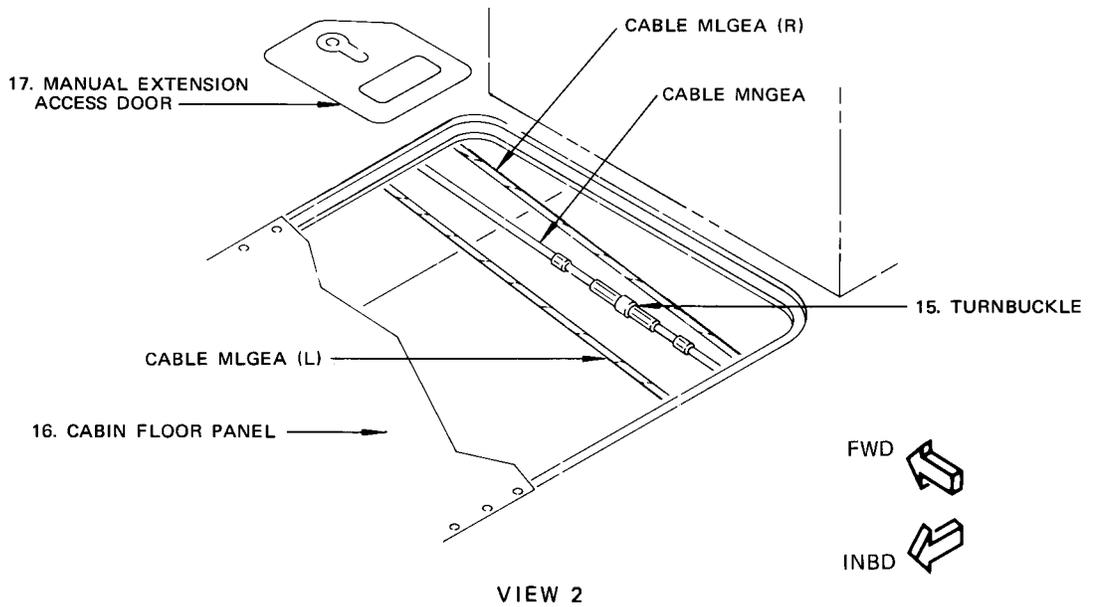
Nose Gear Manual Extension Release Mechanism Installation
