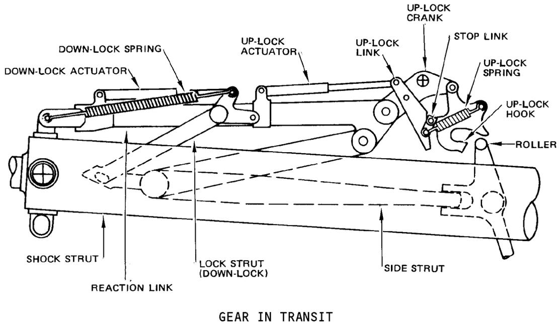
Main Gear Mechanism Schematic
